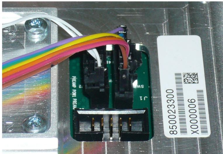
16. Insert the ribbon cable in the connector. Push the cable fully into the socket and listen for a click sound.
