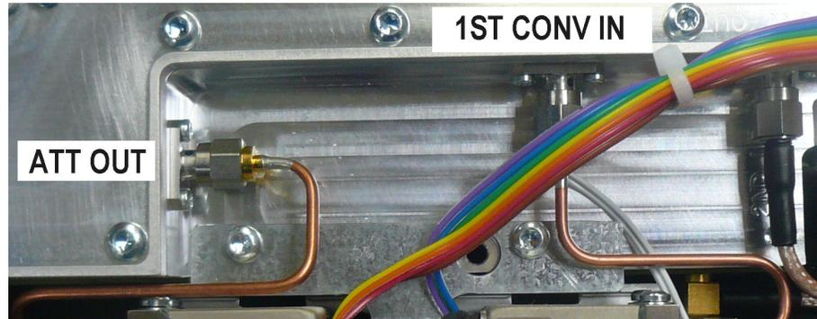
5. Use the two screws, previously set aside, to attach the preamp assembly to the 1st Converter. Do not tighten the screws yet.
