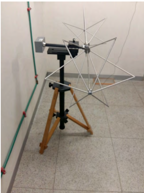
Figure 70: The above image shows the mounted antenna with the pipe holder.
