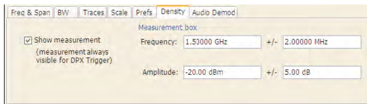
Figure 27: DPX Density control panel is used to define the area of interest for DPX density measurements.
