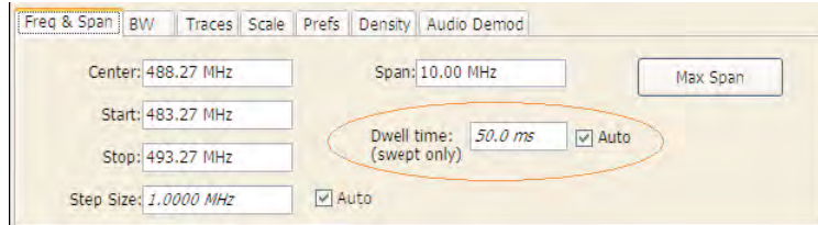
Figure 17: During swept DPX operation, the Dwell time control adjusts the observation time of each frequency segment used to construct the composite DPX display.
