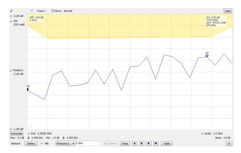
The following figure shows the results of a failing Noise Figure **is outside mask** test with Lower Mask and Upper Mask enabled. The red area highlights the area of failure, which occurs at the lower mask. Markers are also in use.
