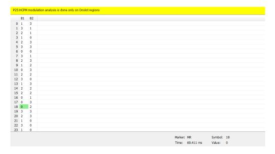
The following image shows the P25 Symbol Table for C4FM (non-bursty) signals. For this signal type and for HDQPSK, there is no grouping into bursts and all symbols that are analyzed are shown.
