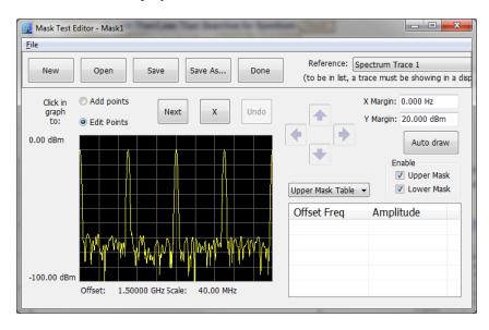
To set up and save mask test limits for a test. Perform the following procedure to set up a test using the mask limits.
