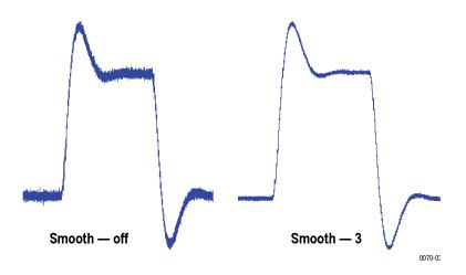
If averaging is turned on, the smoothed data array is averaged with data arrays of previous acquisitions on a point-by-point basis. Smoothing has the advantage of reducing noise-like variations in the measurement, but carries the risk of masking real measurement data. The amount of smoothing applied must be determined by evaluating the waveform you see for artifacts that result from the process.
