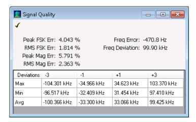
Signal Quality display for nFSK modulation type
