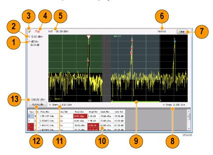
RF Measurements Spurious Display
