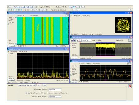
The following screen capture shows the measurement frequency indicator located at 2.0402 GHz while the Spectrum Center Frequency is still located at 2.0000 GHz.
