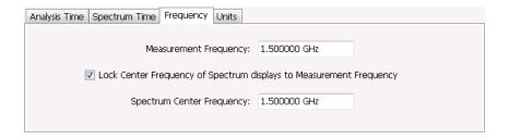
The following screen capture shows a display with both the Measurement Frequency and the Spectrum Center Frequency locked together.
