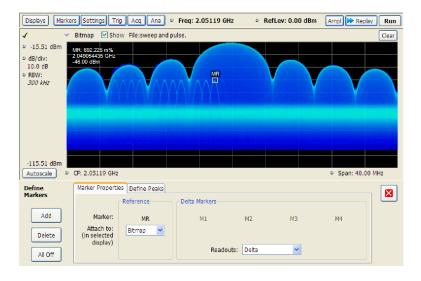
**Searching for peaks on the DPX bitmap trace.** To locate peaks on the DPX Bitmap trace, use the arrow buttons on the Marker toolbar. The left / right arrows move the selected marker to the next peak lower or higher in frequency. The up and down arrows search for peaks at the same frequency. The peaks on the DPX Bitmap trace are defined by the settings for the DPX Signal Density on the Markers > Define Markers > Define Peaks (see page 448) tab.
