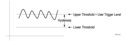
The following figure shows that a trigger is generated when the signal frequency changes sufficiently to exceed the hysteresis value (the difference between the upper and lower thresholds) and cross the lower threshold followed by crossing the upper threshold.
