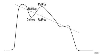
The Ripple measurement, in Watts, is calculated as follows:
