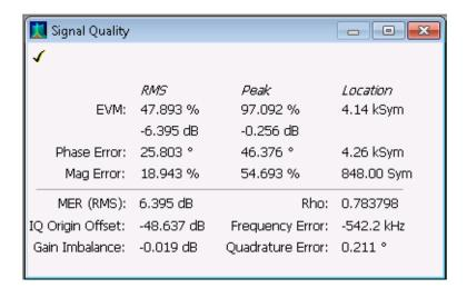
Signal Quality display for all modulation types except nFSK, C4FM, OQPSK, and SOQPSK
