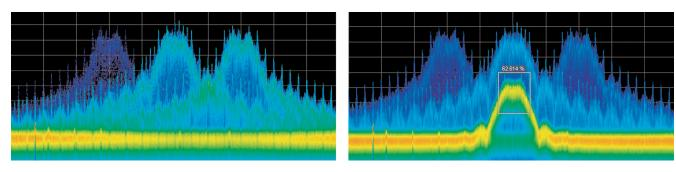
Figure 29. Example of Density Trigger. Left: A free-run DPX display showing pulses with varying frequency. Occasionally, a short pulse in the middle appears for a split instant, but it is hard to capture it with just a Run/Stop button. Right: The triggered DPX displays shows the low-amplitude pulse that was not apparent in the untriggered display. The analyzer was set to trigger whenever the average density in the user-drawn box measured 50% or higher.
