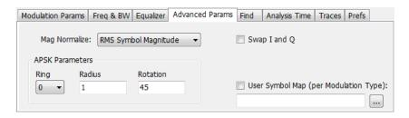
Advanced Params tab for modulation type APSK
