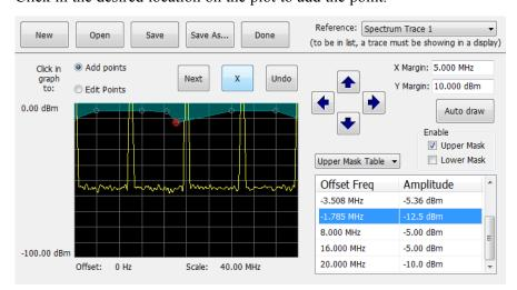
**f.** To use the auto draw feature to automatically place points on the chosen mask, enable the desired mask from the drop-down menu and then click the **Auto draw** button.
