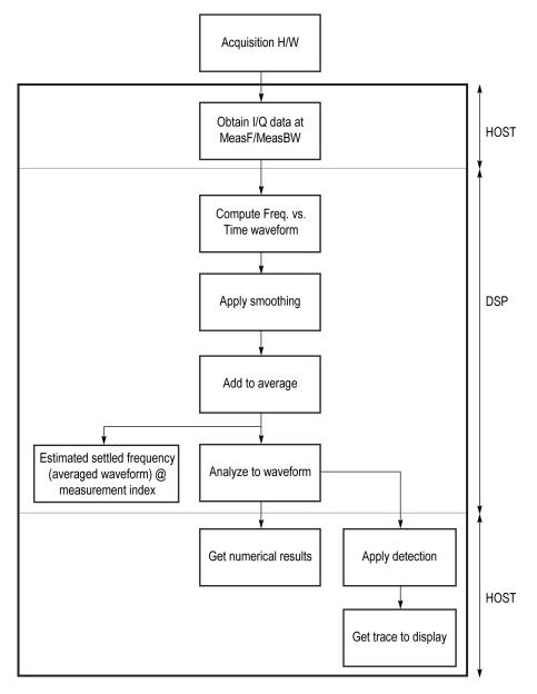
Frequency settling time flow diagram
