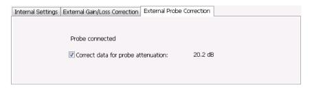
The analyzer can detect when an RTPA2A TekConnect probe adapter is connected to the instrument. The only setting available on the tab specifies whether a correction is applied to the signal or not. The amount of correction is specific to the probe and is communicated to the signal analyzer through the RTPA2A TekConnect probe adapter.
