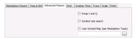
Advanced Params tab for modulation type nFSK
