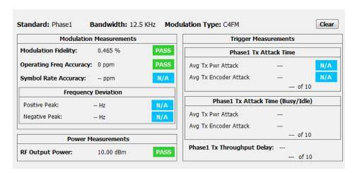
The following image shows an example of the display for a Phase 1 C4FM High Deviation signal.
