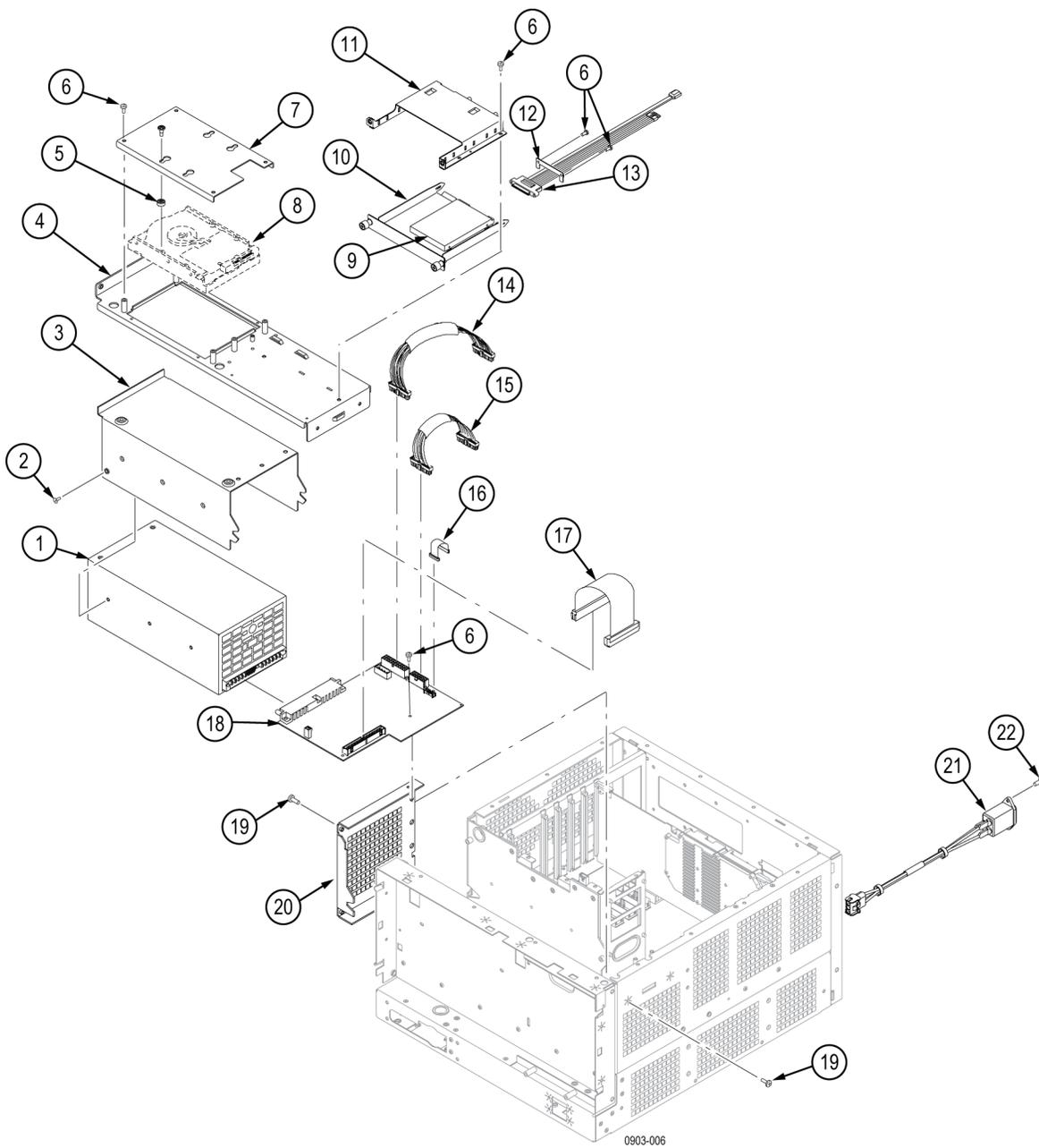
Figure 4-4: Power supply and hard drives
