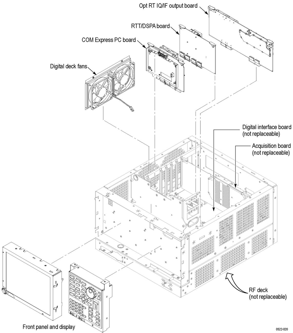
Figure 3-2: Main customer replaceable modules
