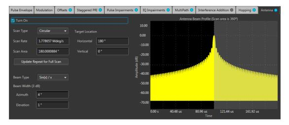
The above image shows settings for the Antenna tab when Circular is the selected Scan Type and Sinc (Sinx/x) is the Beam Type.
