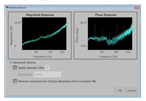
If applying an I/Q correction file (to a pair of I and Q waveforms), the Frequency Response screen shows plot information and provides Advanced options to apply a skew.
