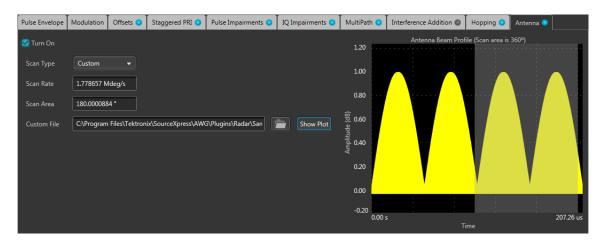
The above image shows settings for the Antenna tab when Custom is the selected Scan Type and Show Plot is selected.
