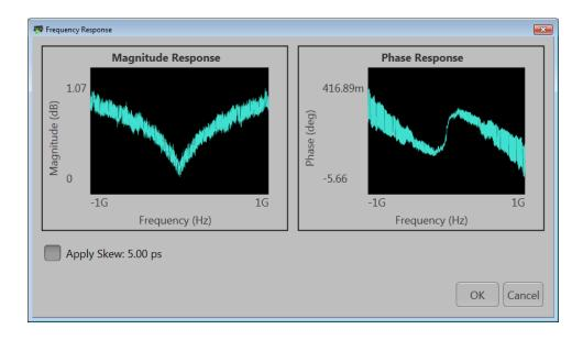
When applying an I/Q correction file you can choose either a single IQ correction file or correction files for I and Q. The Frequency Response screen shows plot information and provides Advanced Options to apply a Gaussian filter or remove Sin(x)/x distortions. When selecting I and Q correction files, separate files for I and Q are shown in the Frequency Response window.
