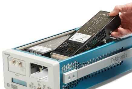
5. Push down lightly on the rear of the module to seat it securely into the mainframe. You will hear a click when it seats fully.
