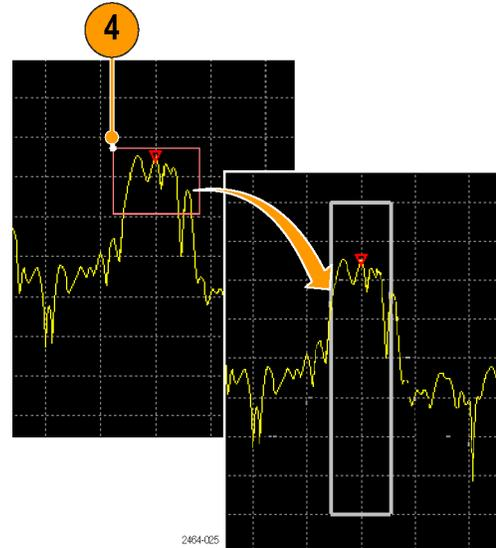
5. Tap the **Region Span** field to enter a precise frequency span of the region.
