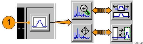
2. To change the width (frequency span) of a region, tap the **Change Span** button.
