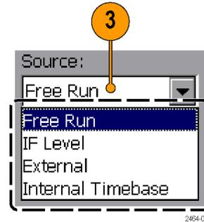
4. Set the trigger parameters. Note that Position is only available when in Amplitude vs. Time measurement mode.
