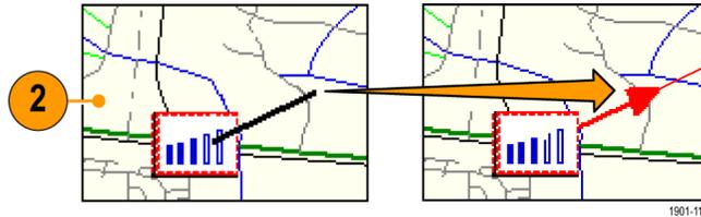
The iMap measurement thumbnail display shows the direction of the arrow as you draw it. The information shown depends on the map type (grid or image). The example shown is for a grid map. Use the thumbnail readout to help set the measurement arrow direction.
