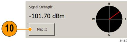
11. Repeat steps 9 and 10 to measure the signal in other directions. Repeat step 10 to take multiple measurements in the same direction.
