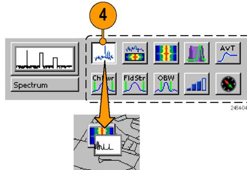
5. To move an icon, tap the **Select** button and then tap and drag the icon to a new position. If the measurement was part of a stack of measurements (such as created by logging), then iMap moves the topmost icon in the stack. If the icon is moved to a new stack of measurements, then the icon is placed in the stack in time-of-measurement order.
