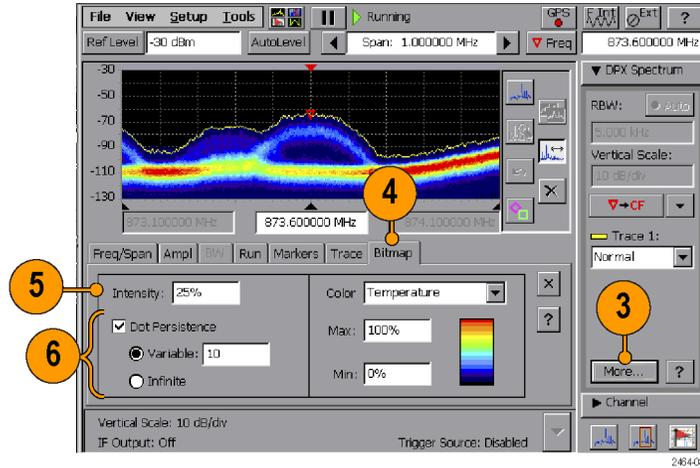
6. Tap the **Dot Persistence** check box to enable Bitmap point display persistence controls. Dot persistence sets how long a point is displayed if it is not updated with new data.
