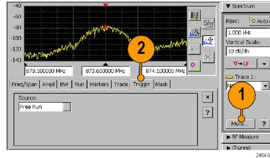
3. Tap the **Source** field and select the trigger type. The External setting requires a TTL-level trigger signal at the Trigger/Timing connector.
