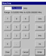
Tap a keypad button to open a keypad in which to enter a value in the selected field. The keypad content changes to show the available entry functions for the selected item.
