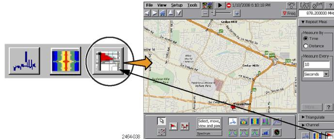
You can load scanned bitmap files as maps for in-building mapping, or use GSF and MIF map file formats for outdoor maps. Using GSF or MIF map files lets you use the built-in GPS receiver to automatically place measurements at your current location.
