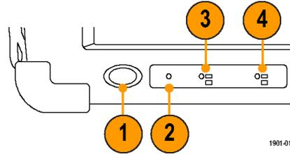
2. Reset button. Performs a hardware reset; all programs and data loaded into volatile memory are erased. Generally only used to recover from a system lock-up. Use a thin probe to push the reset button.
