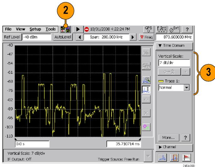
4. Tap the **More** button in the Time Domain drawer to display the spectrum parameter tabs.
