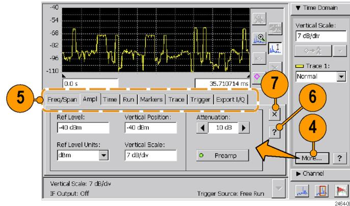
8. Use the **Zoom** and **Pan Display** buttons to display a waveform segment of interest.
