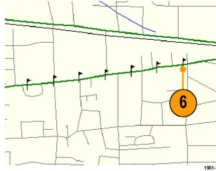
7. Tap the **Single Measurement** or the **Select** button to exit the iMap logging measurements mode.
