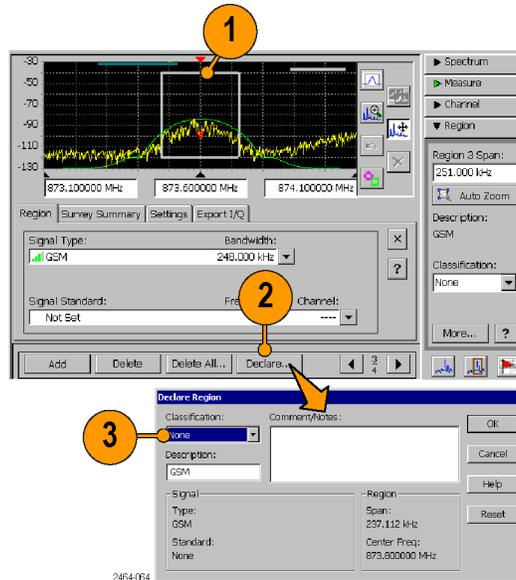
4. Tap the **Description** field to enter a brief description up to 14 characters long. The default value for this field is the signal type as set in the Region tab, but you can change the default value if desired. To enter characters, use the WindowsCE Inputs Panel on-screen keyboard control or a keyboard connected to the instrument PS2 port. (See page 28, *Parameter entry controls*.)
