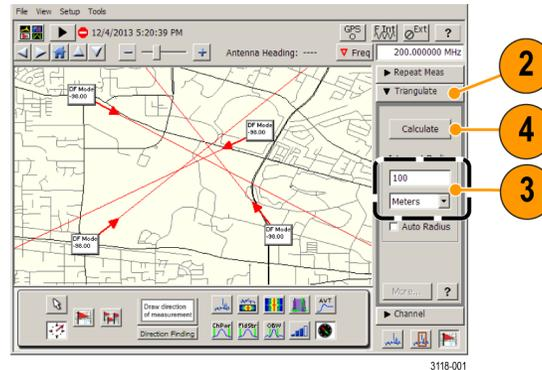
5. iMap draws circles around all intersections that can be enclosed in a circle of the specified radius.
