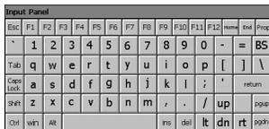
WindowsCE provides an Input Panel (virtual keyboard) that you can use to enter text such as file names. In most cases, when the instrument opens a dialog box that includes fields for text entry, the Input Panel also opens. When you close the dialog box, the Input Panel also closes.
