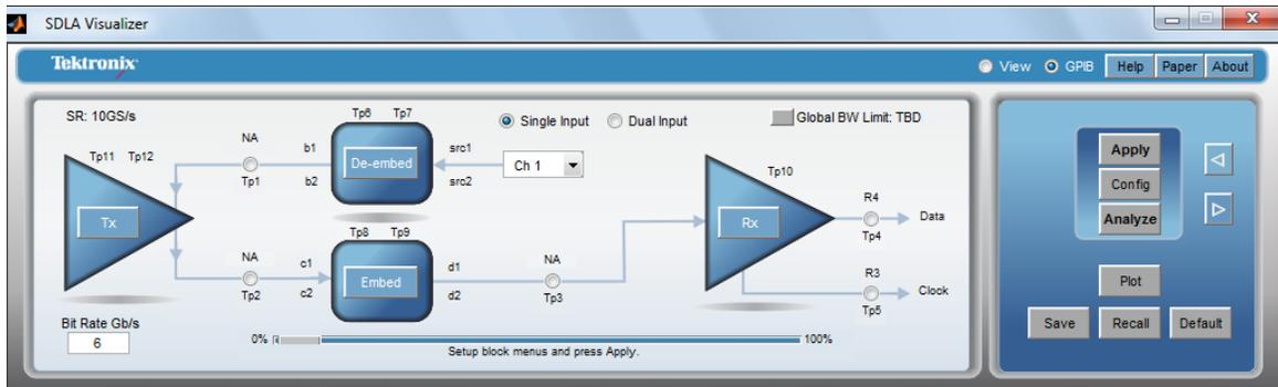
2. The next step is to define the Measurement Circuit model. This is made up of the transmitter source impedance, cable, and scope.
