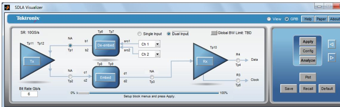
SDLA Visualizer requires you to define two circuit models, the Measurement Circuit and the Simulation Circuit, that both connect to the **Tx Block**. The Tx Block makes use of Thevenin equivalent voltage to provide a point where the acquired waveform is passed into the simulation side of the system. (Thevenin's Theorem states that it is possible to simplify any linear circuit, no matter how complex, to an equivalent circuit with just a single voltage source and impedance.)
