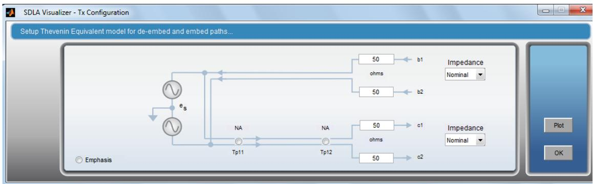
9. Set up the Tx Block to best represent the DUT transmitter source impedance that the system is connected to. Press **OK**.
