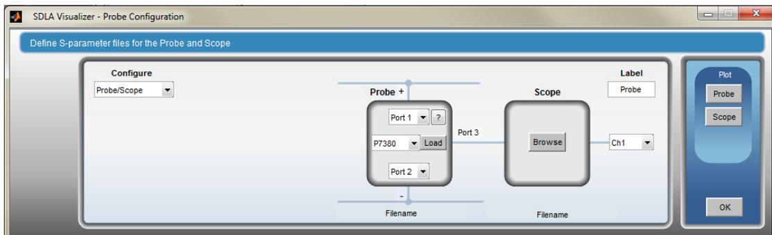
On the **Probe** drop-down menu, choose the correct model that is in use. For example, P7380 was selected in the image above. The browser will then open the correct directory for the selected probe model:
