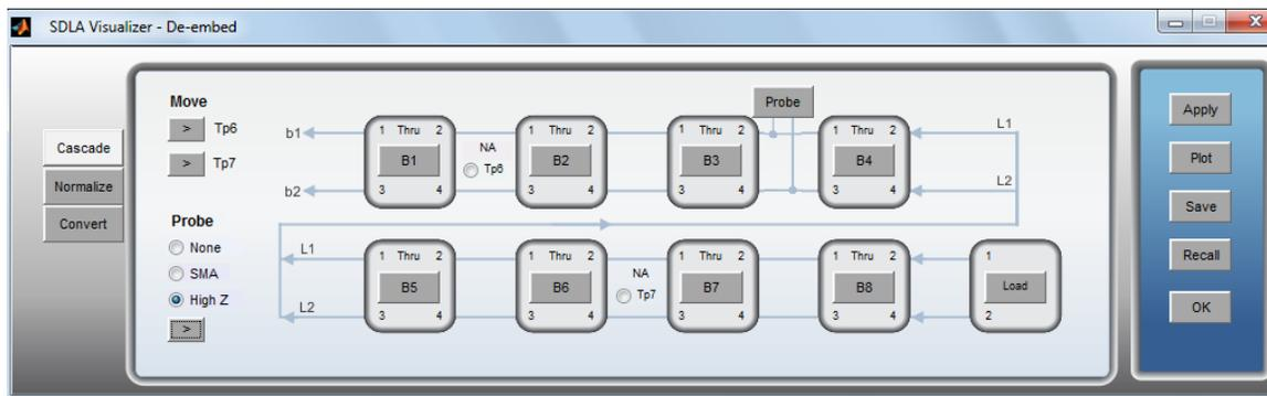
3. Press the **Probe** button. This brings up the Probe Configuration Menu:
