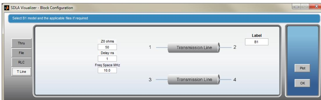
This allows you to define a lossless transmission line. SDLA computes a set of 4-port S-parameters depending on the parameter settings in the edit boxes. The cross-coupling terms shall be set to zero. Press here for more information.
