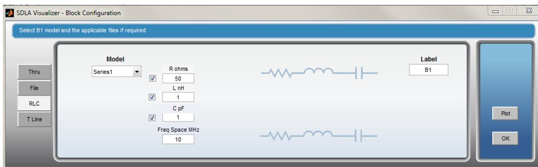
The RLC Tab **Model** drop-down menu offers four different series and shunt configurations of RLC networks. Press [here](#) for more information.
