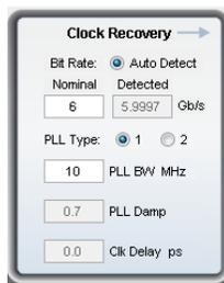
Clock recovery is used for FFE/DFE equalization in the Rx Block. The software performs clock recovery by emulating a phase locked loop (PLL) circuit. Use the data rate defined for the serial standard you are testing. If you are testing a new serial line, you may need to measure the bit rate near the transmitter, or
