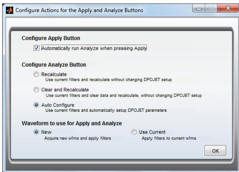
6. Now, process the models by pressing **Apply** on the Main Menu. This will compute the transfer function at **Tp2**. The resulting waveform will be visible on the oscilloscope in Math 1. Since DPOJET was configured to run automatically, DPOJET will setup to measure TIE and plot the Eye Diagram at Tp2.
