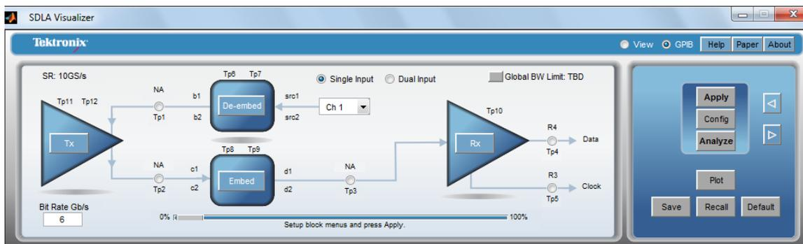
2. This brings up the De-embed Menu. Select the **High Z** radio button. This causes a **Probe** button to appear on the circuit diagram, as well as an arrow that lets you move the location of the probe on the diagram.
