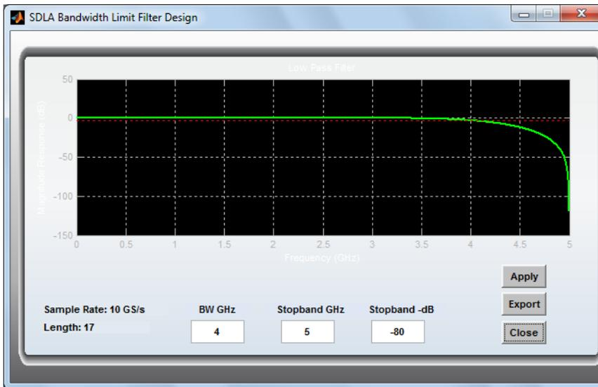
3. Set values in the BW GHz, Stopband GHz and Stopband dB fields.
