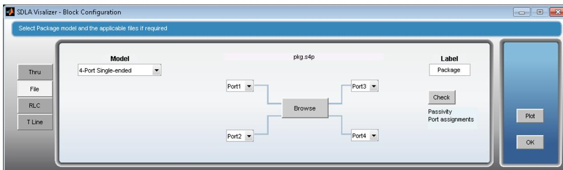
2. To see if the port assignments are correct, you can press the **Check** button located on the **File** tab. You can also check the S-parameter plot to identify insertion loss terms to assign ports properly. Press **OK**.
