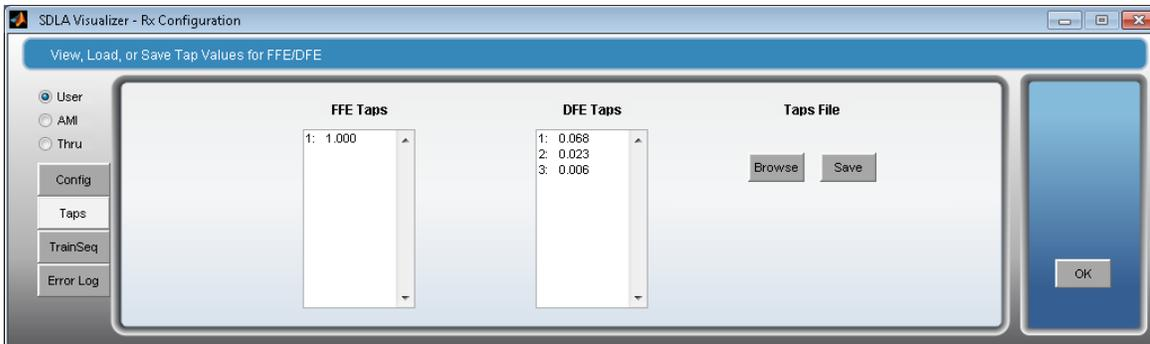
When **PCIE3** is selected in the FFE/DFE panel (in the drop-down menu under **FFE/DFE Type**), and **Auto** or **From Current** is selected under **Adapt Taps**, the DFE adaptation algorithms attempt to maximize the eye area. The resulting DFE tap value is shown in the Taps tab.
