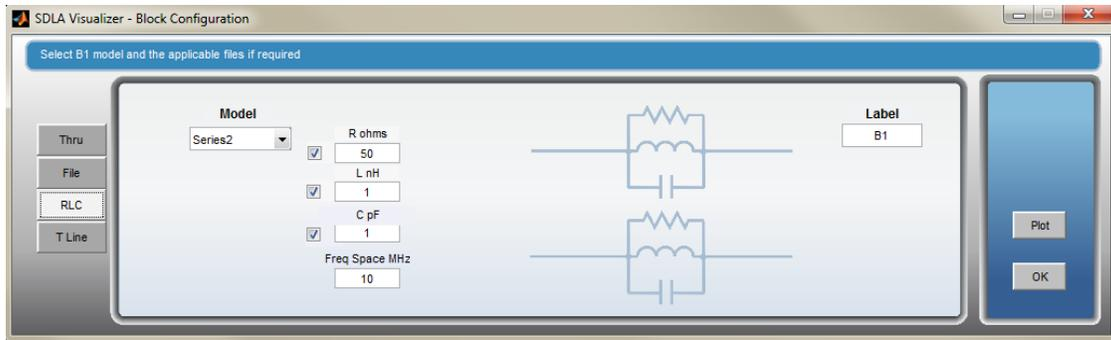
**Shunt 1.** Represents series RLC networks in shunt with each line:
