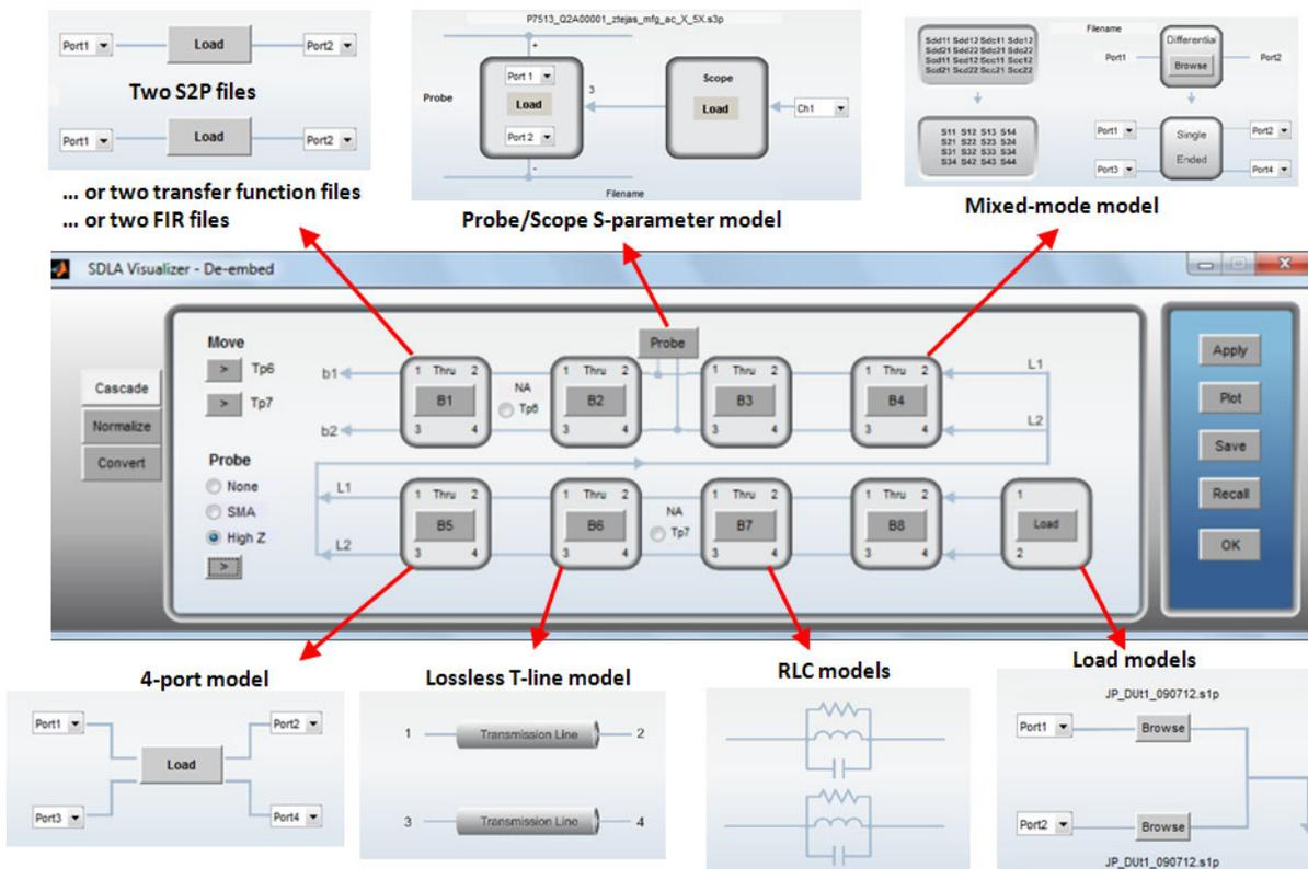
**NOTE.** *If the DUT has large attenuation, de-embedding results will have limited bandwidth, ringing, and slower rise-time. If you increase the bandwidth limit filter transition band, it can reduce ringing at the expense of phase and magnitude error at the higher frequencies, and at the expense of increased noise.*
