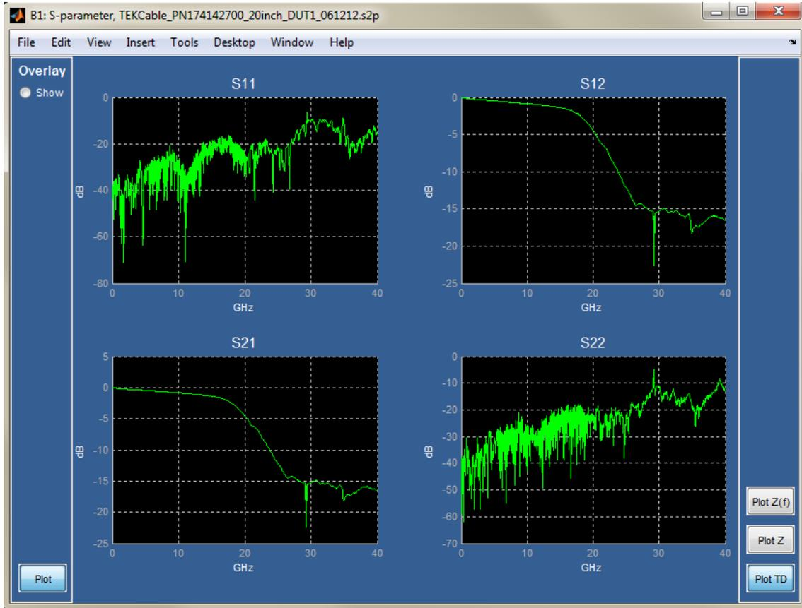
2. Press the **Plot TD** button in the S-parameter plot menu to open another window, shown below, containing the time domain plots for each S-parameter:
