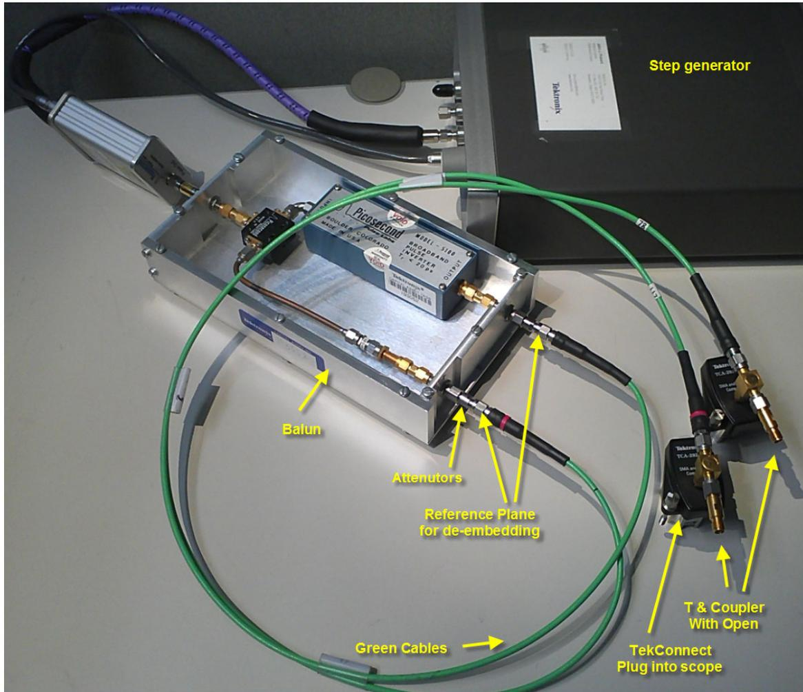
Below, the outputs of the T couplers are connected to the CH1 and CH2 inputs of the oscilloscope:
