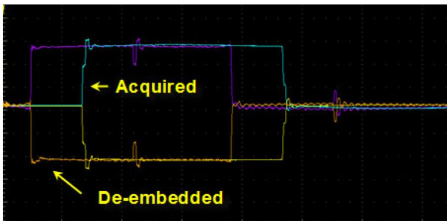
2. The image below shows **Tp2**, which in SDLA is at the output of the Tx model with the embed side of the system loading the Tx model. In this example, Tp2 provides the waveforms with the measured cables and components removed, and the step generator reference plane terminated in an ideal 50 ohms. All blocks were left set to default Thru models, and the load was default 50 ohms.
