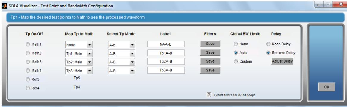
2. Under **Global BW Limit**, select **Custom** and then press **Setup BW**. This brings up the **Bandwidth Limit Filter Design Menu**.
