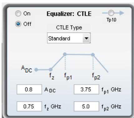
Turn CTLE on or off using the radio buttons on the left. Four CTLE types are available on the drop-down menu:
