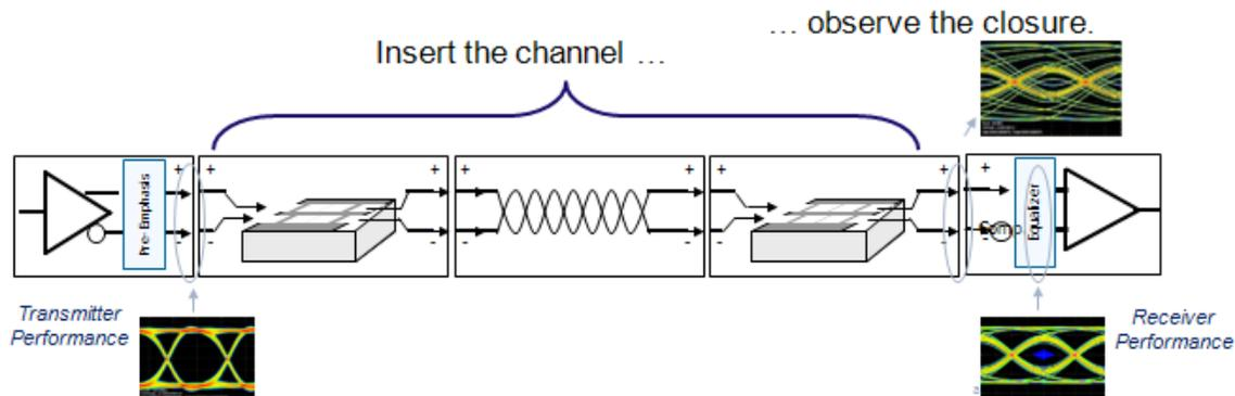
Create a simulated channel to embed by pressing **Embed** on the Main Menu. This brings up the Embed Menu. Using this, you may configure the blocks in many ways. Press here for some possible configurations. For more information, see [De-embed/Embed Menu \(see page 32\)](#).
