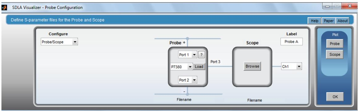
4. In the **Probe** panel, select the correct probe model. Press **Load** to bring up the probe browse menu, and load the 3-port S-parameter file.
