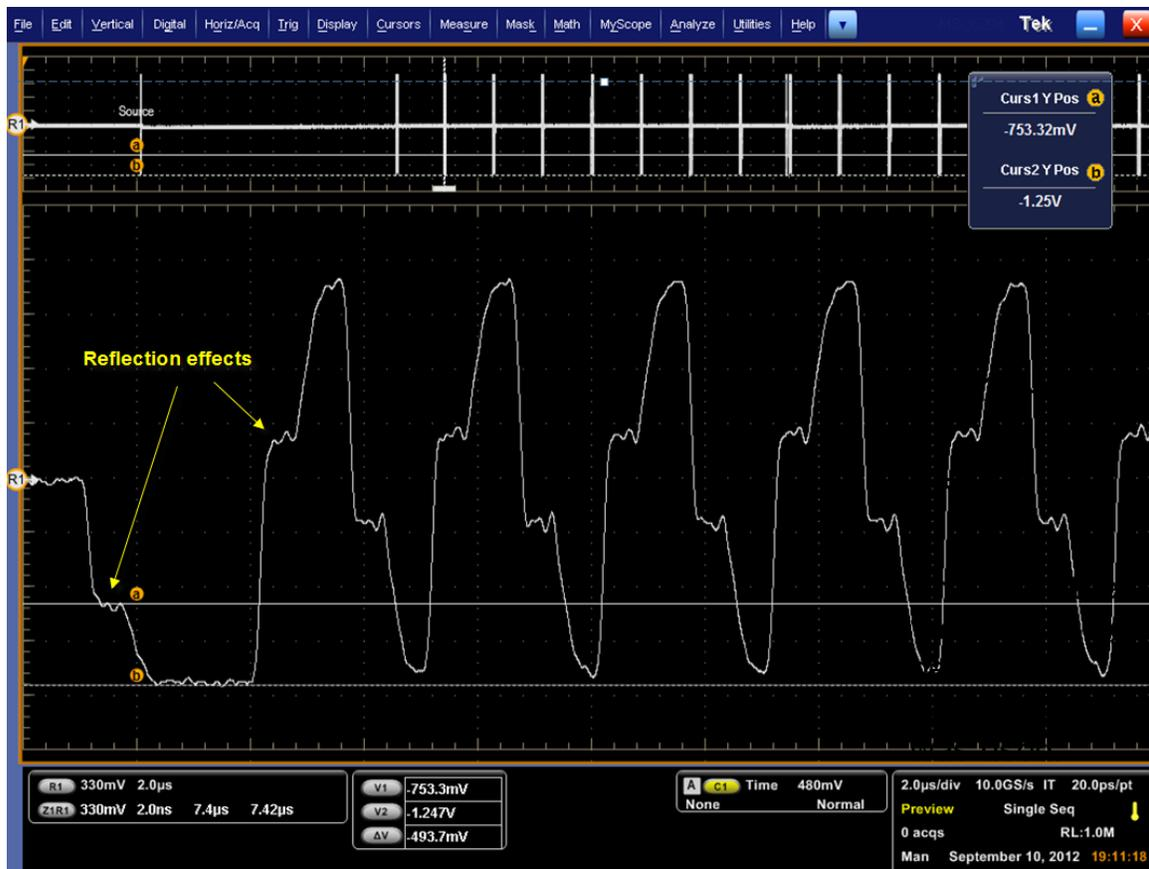
Even though the waveform at the actual probe point is not suitable for any jitter measurements due to the large reflection, the waveform at the load resistor has a regular pulse shape. This example shows how SDLA can be set up to de-embed the reflection from the waveform at the load resistor.
