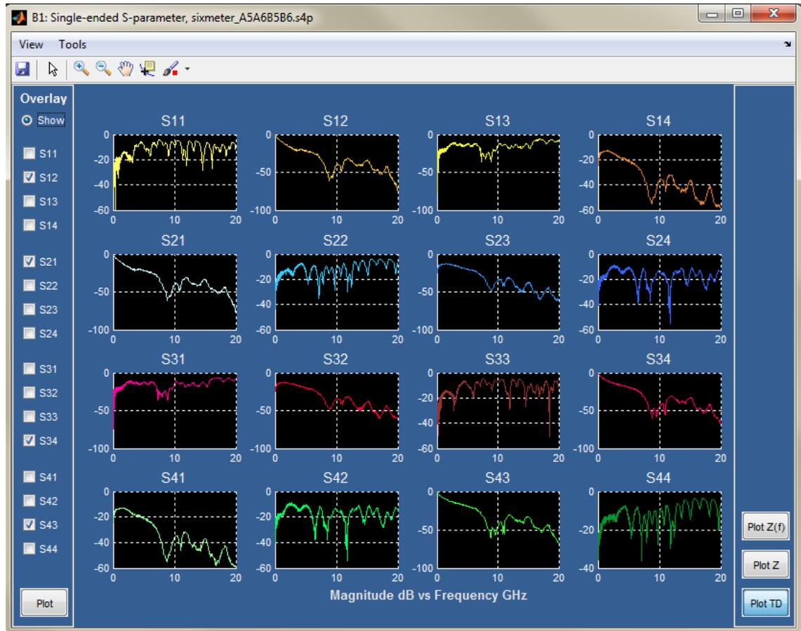
The **Overlay Menu** is on the left side, with a **Plot** button at the bottom. Pressing **Plot** opens a window with four overlaid axes: dB vs. GHz, Phase in Degrees vs. GHz, Amplitude vs. Time, and Step Response vs. Time.
