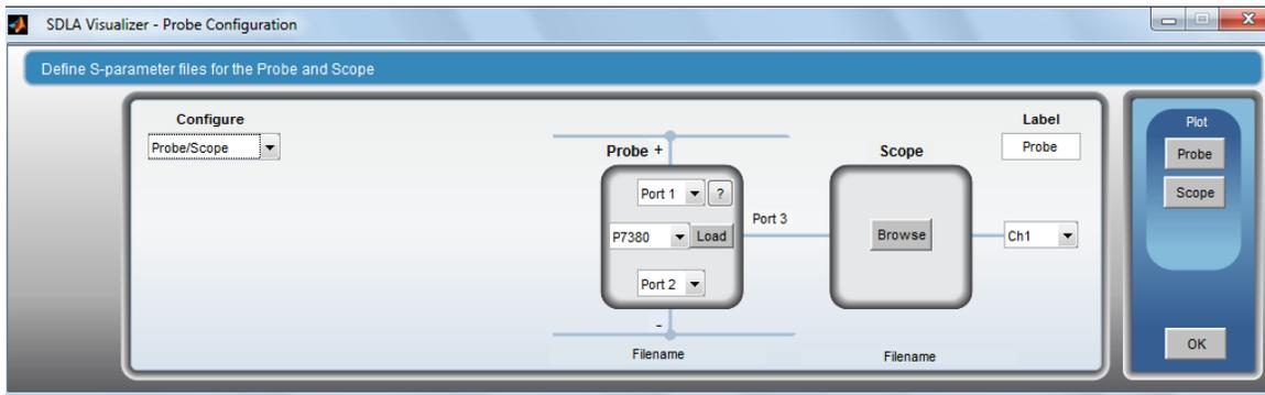
Under **Configure**, select the circuit configuration desired. There is choice of **Probe/Scope**, shown above, or **Interposer/Probe**, shown below:
