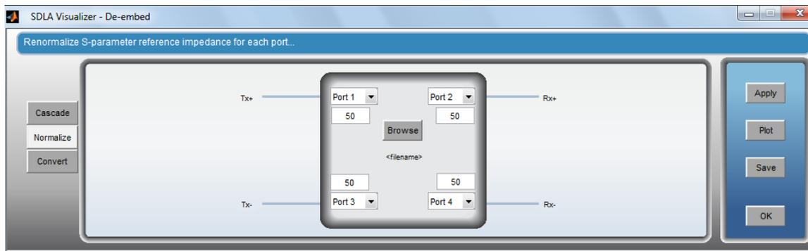
3. Touchstone 1.0 format only supports one impedance value for all ports. That number will be displayed in the port edit boxes. Now, edit each box to 50 Ohms for internal use with SDLA. Edit any port to desired values for external use outside of SDLA or for observing differences in the plots.
