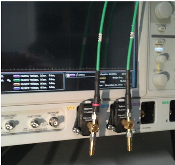
In order to provide a set of S-parameters that SDLA Visualizer modeling blocks can use to create real-time waveforms, the 2-port S-parameters for each cable and for each T coupler combination were measured on a VNA.
