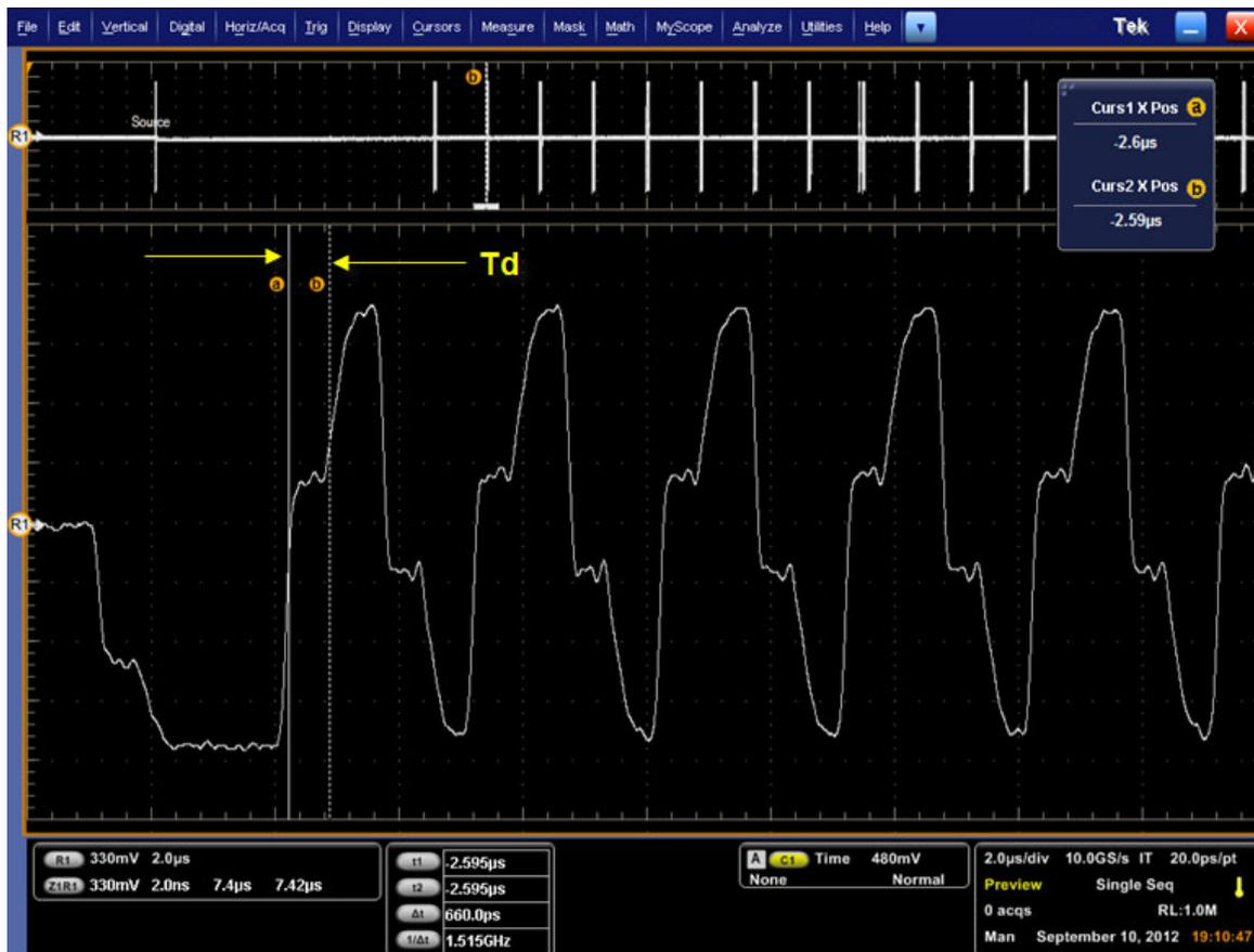
2. Set up a block using a lossless transmission line model with 330ps delay. Select block **B2** in the **De-embed** menu and select the **T-line** tab. Enter 0.33 in the **Delay ns** field. Press **OK**.
