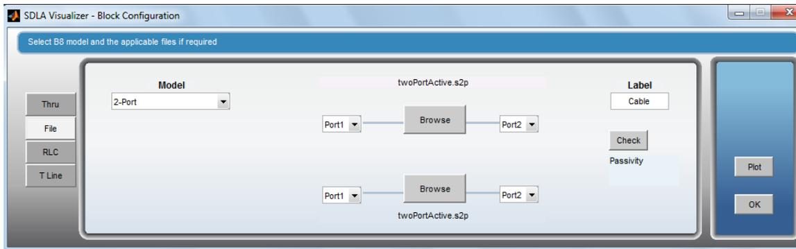
3. The next step is to define the Simulation Circuit model. In this example, we will drive the transmitted signal into an ideal 50 Ohm load.
