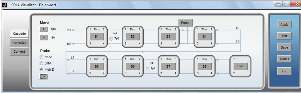
Pressing the **Probe** button on the Cascade Tab diagram brings up the Probe Path Configuration Menu:
