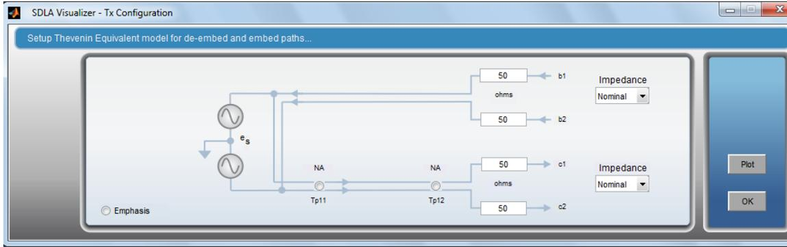
The following image represents the transmitter as one 2-port S-parameter model in the lower (embed) part of the systems, and two 1-port S-parameter blocks in the upper (de-embed) part of the system. These are shown differently to illustrate the choices; normal usage is for both the upper and lower sections to be set up as identical to each other.
