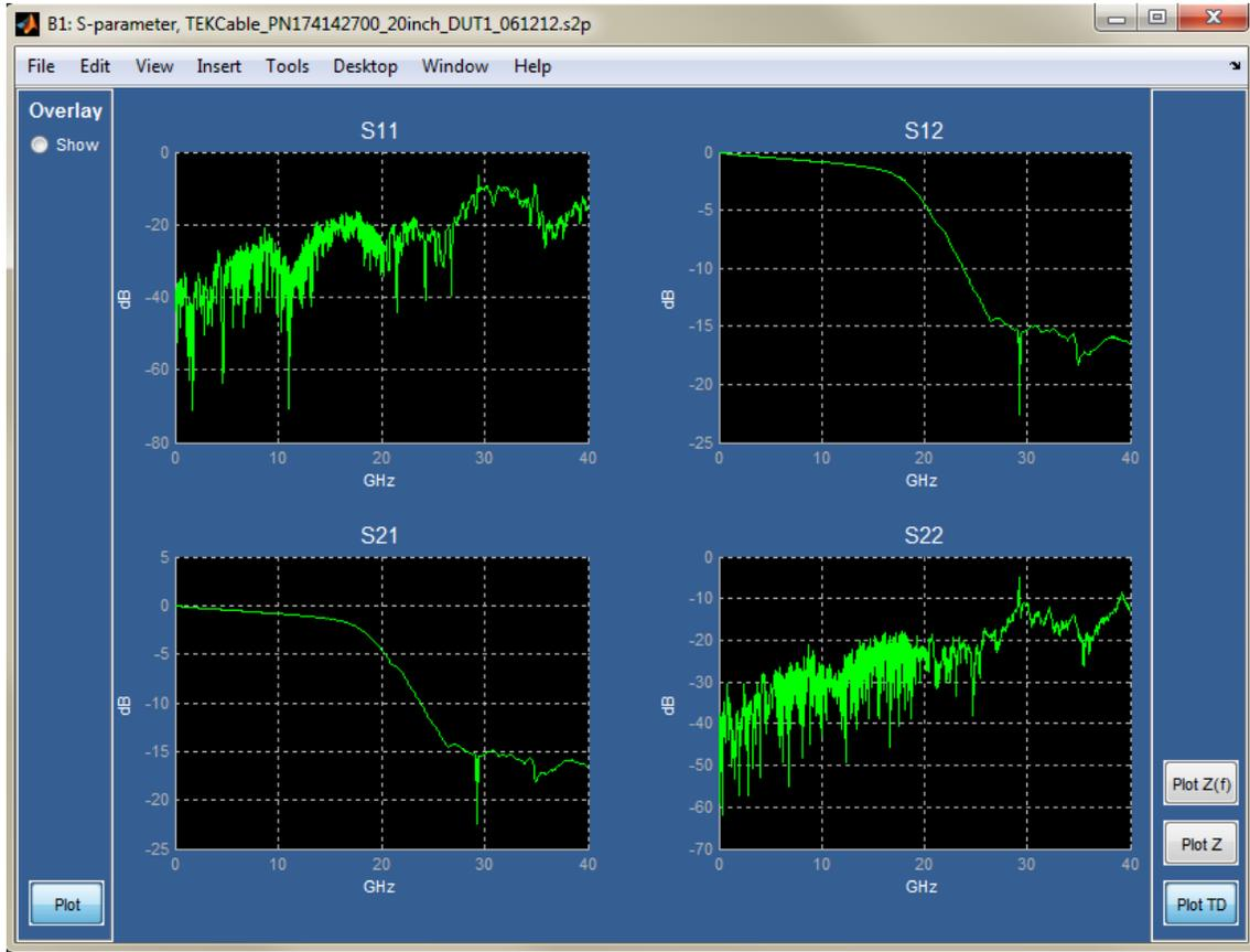
4. At the bottom of the Overlay panel, select **Plot**. This brings up another window, shown below, that contains the overlaid plots. These show magnitude, phase, impulse and step response for the various S-parameters:
