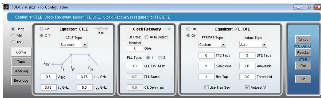
User Mode gives you access to equalization tools and options for recovering the data stream and clock by correcting for the effects of insertion loss, cross talk, reflection, and noise. Many **CTLE**, **clock recovery** and **FFE/DFE** parameters can be specified, plus Taps definition and training sequence detection. This mode also implements the behavioral equalizers of PCI Express, Gen3, SAS 6G, USB3, etc.
