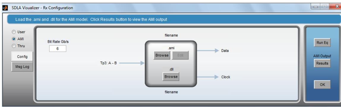
To use AMI Mode, from the Rx Configuration Menu select the **AMI** radio button and press **Browse** under .ami. On the resulting menu, select the .ami file you'd like to use. Press on the lower **Browse** button to select the .dll file you'd like to use.
