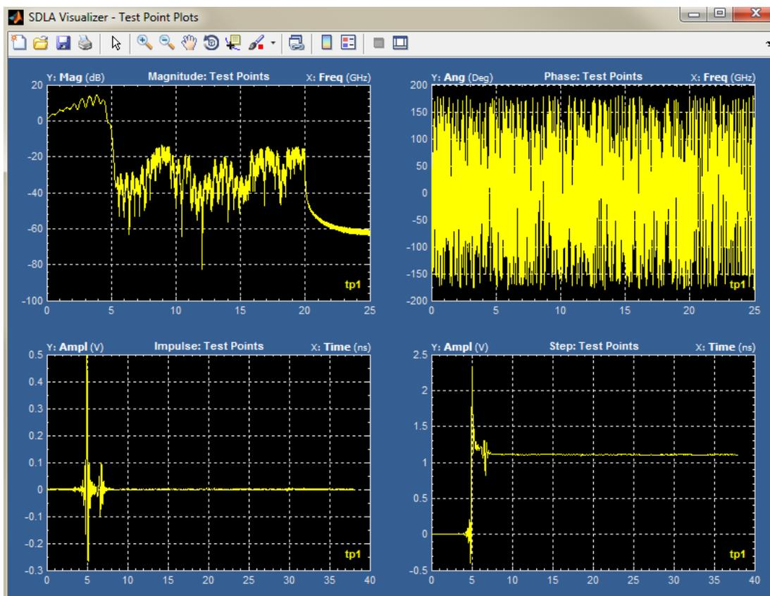
**Global Bandwidth Limit.** This allows you to set up how the global BW limit filter will be applied to all test point waveforms. Under the **Global Bandwidth Limit** label, three options are available, including the option to create a custom filter. Press here for more information..
