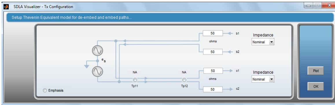
**NOTE.** The impedance value should model the actual impedance of the transmitter. This can be done using either actual S-parameters or nominal values. It is important that this value match the transmitter impedance for the most accurate de-embedding.
