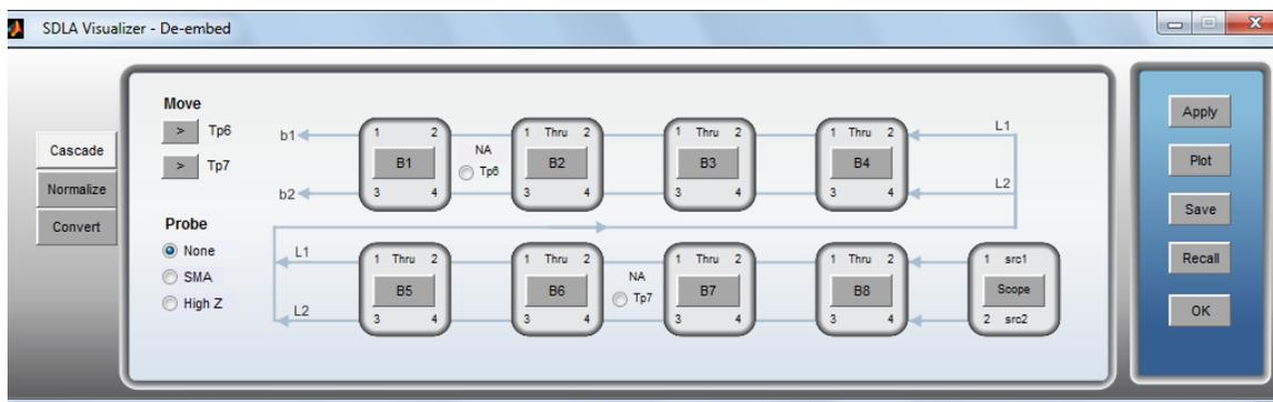
Pressing **De-embed** on the Main Menu brings up the De-embed Menu; pressing **Embed** brings up the Embed Menu. These menus display a diagram of 8 cascaded 4-port S-parameter block models, plus a load model at the end, which you may configure, plot and save. You may also select the locations of two movable test points, configure the load, and configure probes (de-embed menu only).
