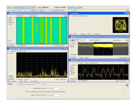
The following screen capture shows the measurement frequency indicator located at 2.0402 GHz while the Spectrum Center Frequency is still located at 2.0000 GHz.
