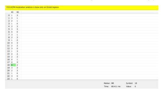
The following image shows the P25 Symbol Table for C4FM (non-bursty) signals. For this signal type and for HDQPSK, there is no grouping into bursts and all symbols that are analyzed are shown.
