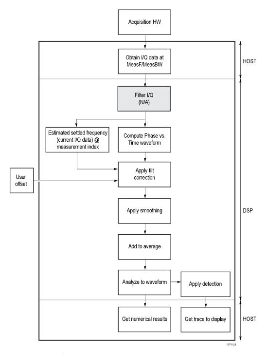
Phase settling time flow diagram
