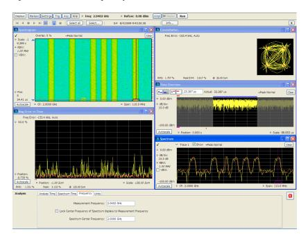
You can drag the Measurement Frequency indicator on the screen to set the measurement frequency. Note the base of the Measurement Frequency indicator. The width of the box indicates the widest measurement bandwidth in use among the open displays. You can see how the width of this box changes with the measurement bandwidth by, in this example, adjusting the Measurement BW setting for the Constellation
