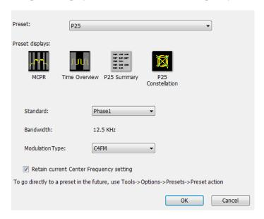
The default adjacent channels table for MCPR is different for RF frequencies in the range of 769 to 806 MHz (called 700 MHz band) and for frequency ranges outside it. The option of retaining center frequency in Standards Preset is therefore useful if you want to load the default table for center frequencies in the 700 MHz band.
