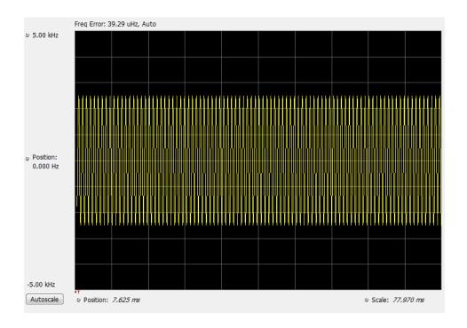
The following image shows the P25 Freq Dev vs Time display for Phase 2 HCPM (bursty) signals.
