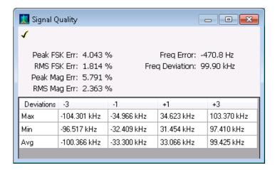
Signal Quality display for nFSK modulation type
