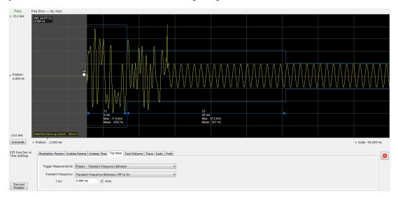
**HCPM Tx Logical Channel Time Alignment (Phase 2 HCPM).** The following information is specific to this measurement. This result can be viewed in P25 Summary and P25 Power vs Time displays.
