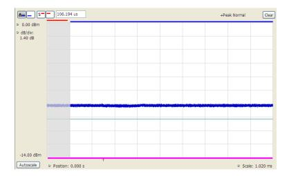
Setting the starting point of the settling time measurement
