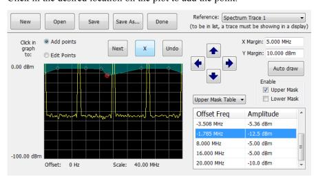
**f.** To use the auto draw feature to automatically place points on the chosen mask, enable the desired mask from the drop-down menu and then click the **Auto draw** button.
