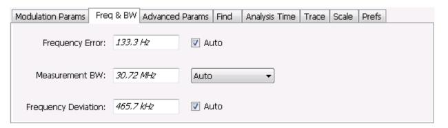
Freq & BW tab with nFSK or C4FM modulation type selected and Frequency Error readout enabled (Auto selected)
