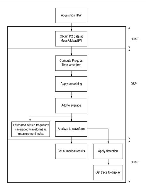
Frequency settling time flow diagram
