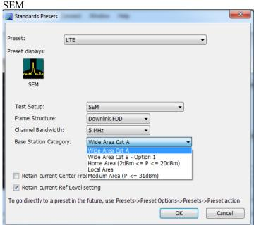
The following table shows what automatically loads with each test setup.
