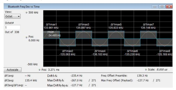
The following image shows the frequency deviation of the first octet in the payload of a Basic Rate signal (low deviation).
