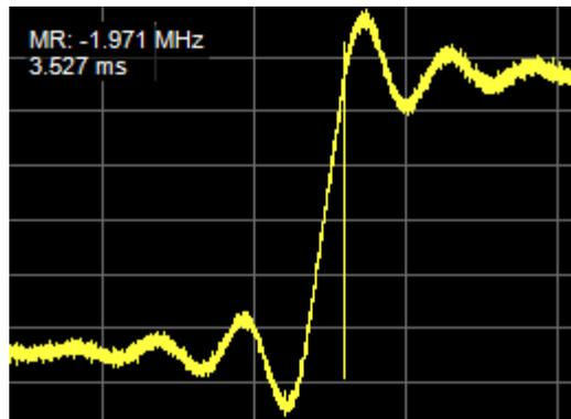
**NOTE.** To optimize the measurement even further, you can go back to step 9 and use the right-button, mouse-controlled **Span Zoom** and **CF Pan** features of the Spectrogram display instead of the **Zoom** and **Pan** features. Then use **Replay** and **Autoscale**. Such an approach might yield a further reduction of the span setting and thus an even cleaner signal on which to make your measurement.
