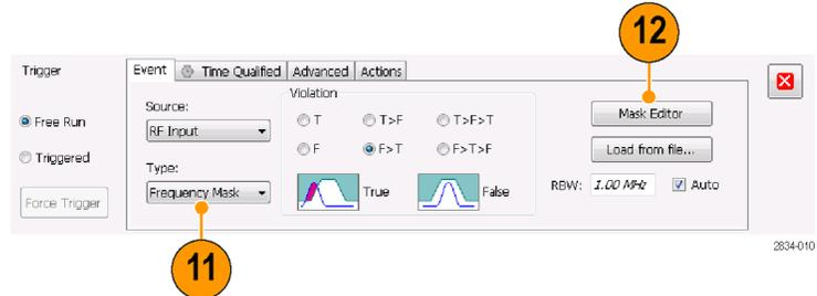
13. Use the Mask Editor to create a mask for your signal. Start by using the **Auto draw** function and adjust if necessary. Traces that you selected in the Spectrum Analyzer display are used as references in the Mask Editor. All trace detections and functions are available.
