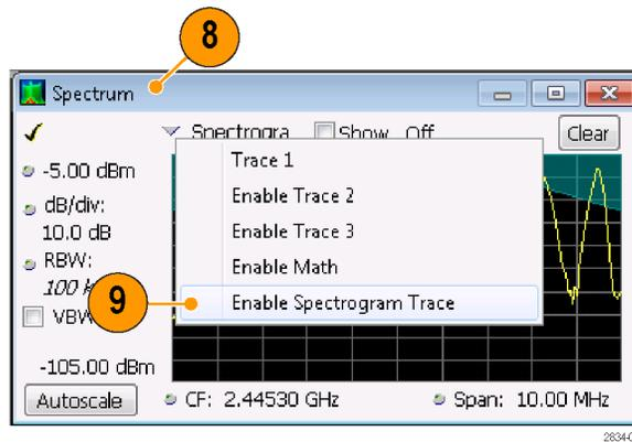
The Spectrogram trace in the Spectrum display corresponds to the line selected in the Spectrogram display by the active marker.
