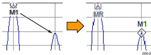
The marker readout at the upper right shows the frequency and amplitude differences between the reference marker **MR** and the **M1** delta marker.
