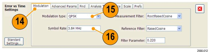
17. Set the Measurement Filter to Root Raised Cosine.
