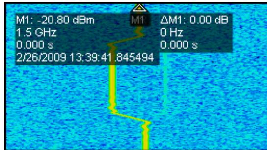
10. Right click the mouse and select **Zoom** from the resulting menu. Pull the mouse vertically and horizontally to zoom in on one or two hops of the spectrogram signal.
