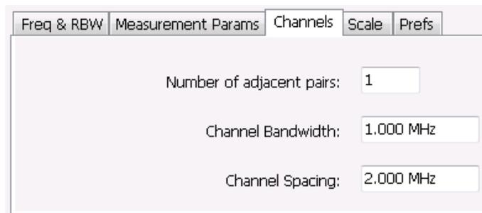
17. Change the **Number of adjacent pairs** to **1**. This will set the instrument to measure the main channel and the one adjacent channel on each side of it.
