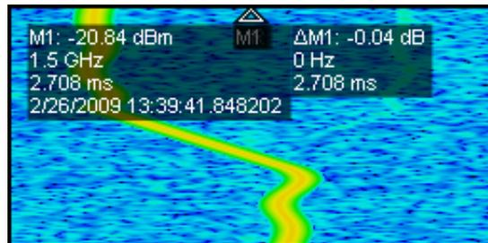
11. Use the mouse to move the MR marker in the *Spectrogram* display to a point of interest. As you move the marker up and down, look at the corresponding changes in the marker in the *Spectrum* display. The *Time-Frequency Analysis* application preset configured the *Spectrum* display to show the selected spectrogram line.
