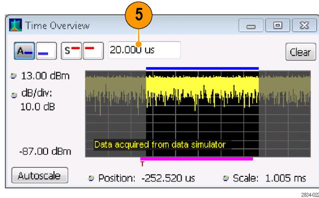
7. Increase the analysis offset again. Because the instrument is stopped, it cannot run a new acquisition to capture a longer data record. When the requested analysis period extends past the end of the data record, the actual analysis length is reduced.
