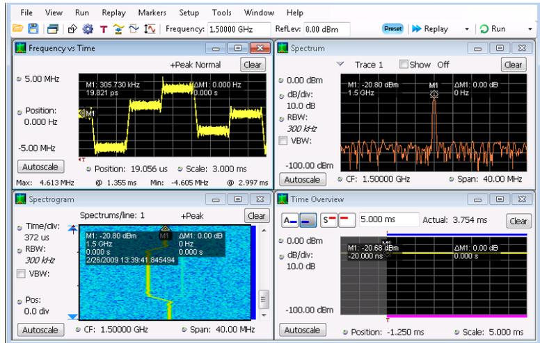
The *Frequency vs Time* display shows the deviation from the center frequency value on the vertical axis and time on the horizontal axis.
