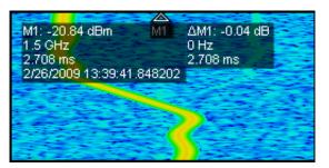
11. Use the mouse to move the MR marker in the *Spectrogram* display to a point of interest. As you move the marker up and down, look at the corresponding changes in the marker in the *Spectrum* display. The *Time-Frequency Analysis* application preset configured the *Spectrum* display to show the selected spectrogram line.
