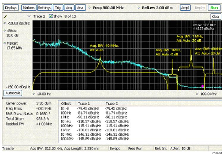
In the previous illustration, the effect of choosing ‘optimize dynamic range’ is seen. In the offsets between 10 Hz and 1 MHz, the 40 MHz acquisition bandwidth is used, and the RF attenuator is set based on the reference level of the instrument to prevent overload of the RF/IF signal path.
