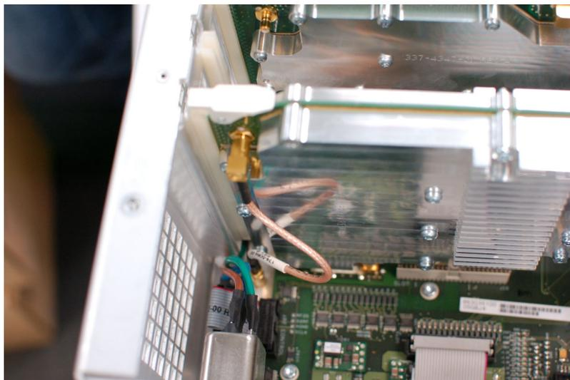
4. If Options 65, 66, or 6566 is installed, reconnect the cabling from this option board, in Slot 3. (See Figure 2.)
