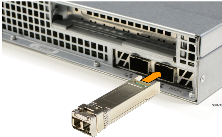
Figure 5: Installing an SFP module
