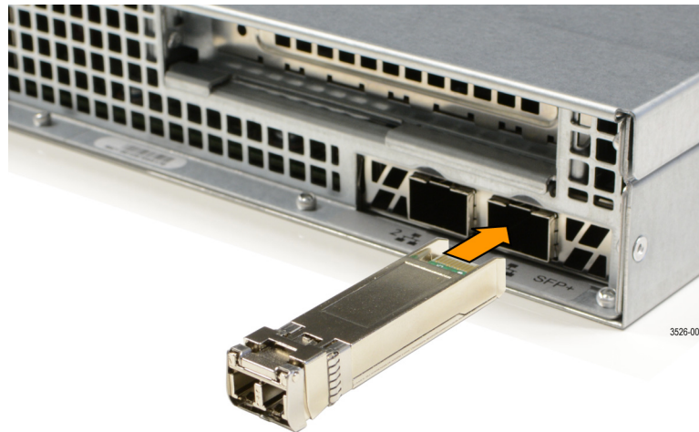
Figure 7: Installing an SFP module
