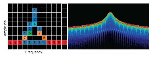
Figure 9: Color-coded low-resolution example (left) and a real DPX display (right).
