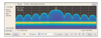
Figure 24: The marker was positioned by selecting the Peak button. Density, frequency, and amplitude measurements at the marker are displayed in the upper left corner of the graph.
