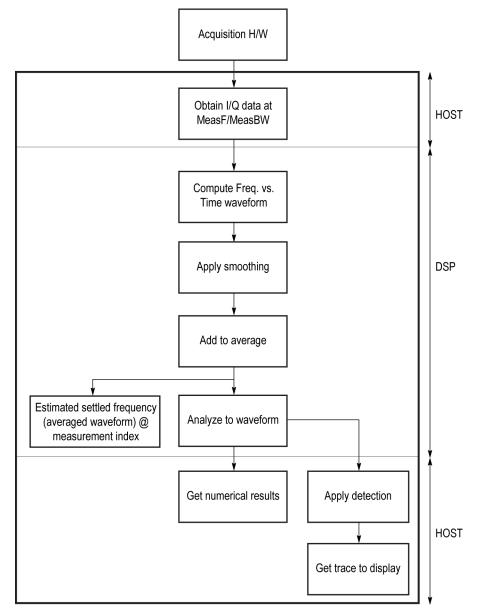
Figure 40: Frequency settling time flow diagram
