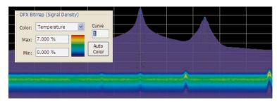
Figure 13: Over a narrow Signal Density range, the color curve is set to 1.
