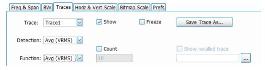
Figure 33: Traces tab with Trace1 and average selected
