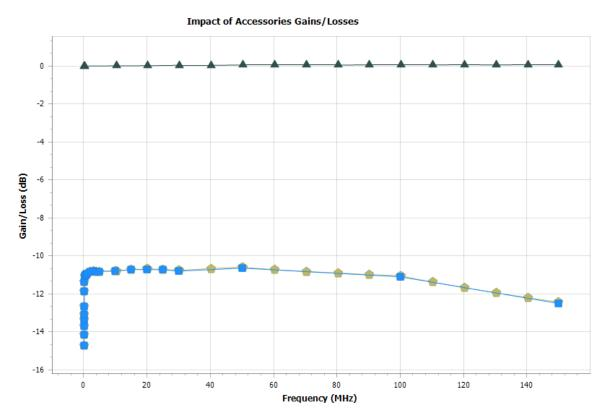
Figure 89: Individual contribution and combined Gain/Loss factors of LISN and a cable (for conducted emission) are shown in the above plot.
