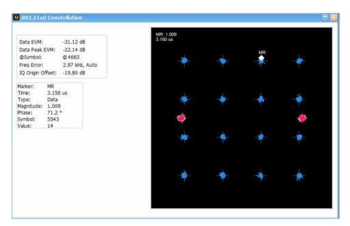
Figure 54: The above image shows an 802.11ad signal with 16QAM data region
