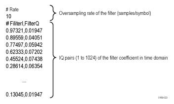
Figure 107: User filter file structure
