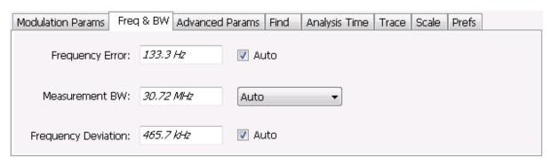
Figure 98: Freq & BW tab with nFSK or C4FM modulation type selected and Frequency Error readout enabled (Auto selected)
