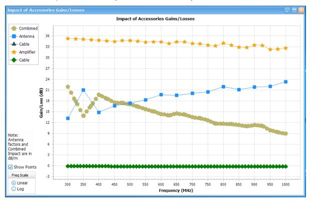
**Antenna factors are used to adjust the final reading as follows.** Corrected Reading (dBuV/m) = Spectrum analyzer Reading (dBuV) + Antenna Factor (dB/m)
