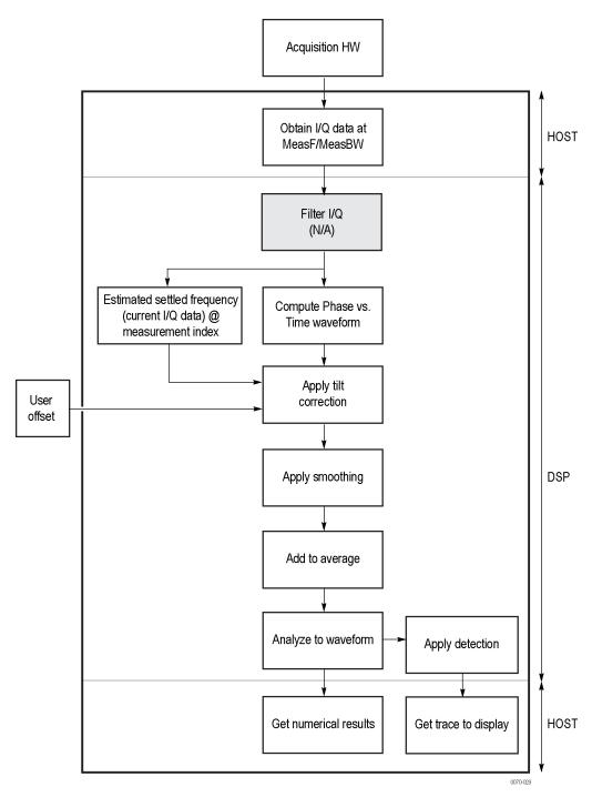
Figure 41: Phase settling time flow diagram
