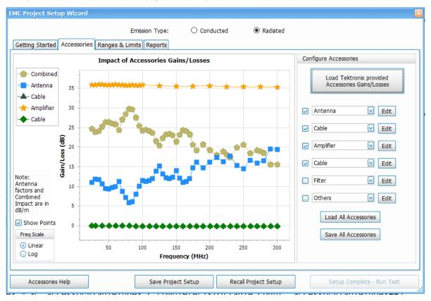
Figure 88: Individual contributions from Antenna, Amplifier, and Cable, and the combined impact, are shown in the above plot.
