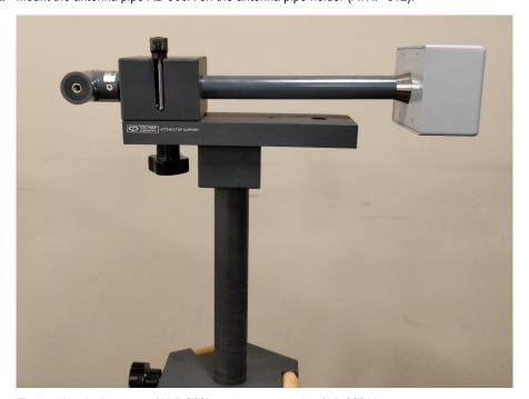
3. Fix the biconical antenna (ABF-900) to the antenna pipe (AB-900A).
