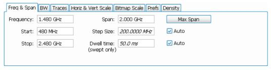
Figure 17: During swept DPX operation, the Dwell time control adjusts the observation time of each frequency segment used to construct the composite DPX display.
