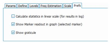
Figure 83: The above image shows the Prefs tab for the Pulse Statistics display when Time Trend is the selected plot type. Trend and FFT plot types do not show the Show Marker readout selection.
