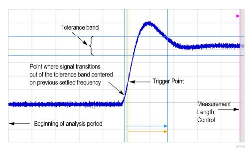
Figure 42: Settling time start reference points
