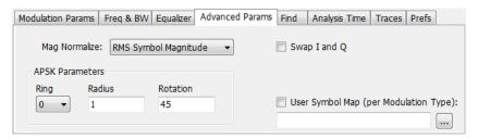
Figure 103: Advanced Params tab for modulation type APSK
