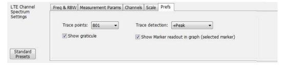
The following image shows the Prefs tab for the LTE Power vs Time display.
