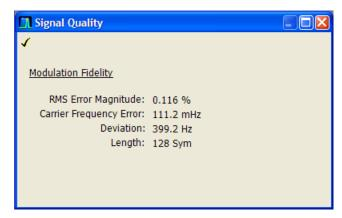
Figure 97: Signal Quality display for C4FM modulation type
