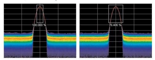
Figure 26: Density of signals defined within an area. Left: Correct measurement of a CW signal. All columns in the box include the signal. Right: Incorrect measurement area. The measurement is accurate, but probably not what you expected. Some columns in the box contain no hits, so they contribute zeros to the calculation of average density.
