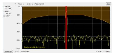
The following figure shows the results of a passing Noise Figure is outside mask test with Upper Mask enabled. Markers are also in use.
