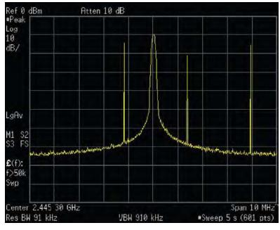
Figure 18: Swept spectrum display of the infrequent transient.
