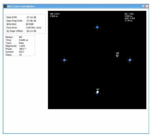
Figure 53: The above image shows an 802.11ad signal with QPSK data region
