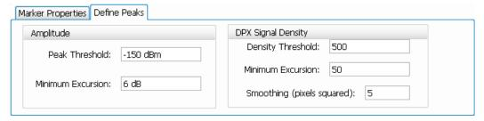
Figure 25: Amplitude and Signal Density controls can be adjusted to define Peak search behavior.
