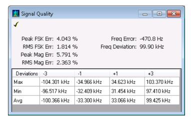
Figure 96: Signal Quality display for nFSK modulation type
