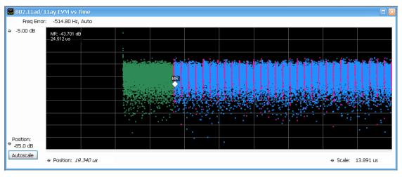
Figure 56: The above image shows a 802.11ay 4.32 GHz pre-EDMG region. The initial empty portion is for the pre-EDMG region.
