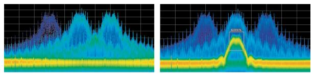
Figure 31: Example of Density Trigger. Left: A free-run DPX display showing pulses with varying frequency. Occasionally, a short pulse in the middle appears for a split instant, but it is hard to capture it with just a Run/Stop button. Right: The triggered DPX displays shows the low-amplitude pulse that was not apparent in the untriggered display. The analyzer was set to trigger whenever the average density in the user-drawn box measured 50% or higher.
