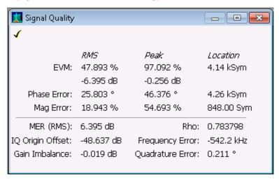
Figure 94: Signal Quality display for all modulation types except nFSK, C4FM, OQPSK, and SOQPSK
