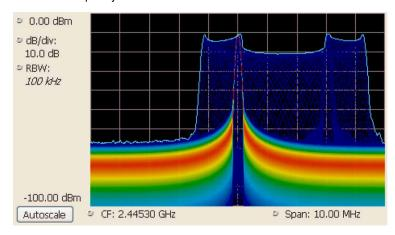
Figure 19: The DPX spectrum display after 5 seconds. The MaxHold trace is cyan.
