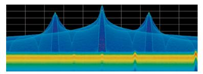
Figure 11: The Auto Color function optimizes the color scale settings
