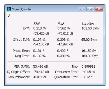
Figure 95: Signal Quality display for OQPSK and SOQPSK modulation types
