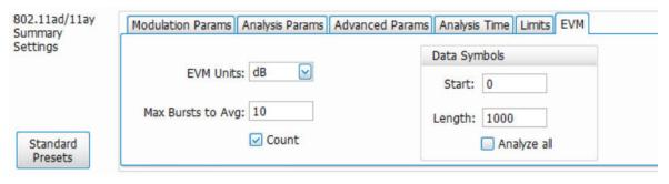
Figure 61: The above image is the EVM tab for the 802.11ad/11ay Summary display for 802.11ad Single Carrier
