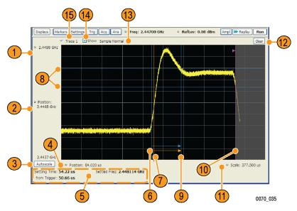
Figure 43: Frequency settling time display
