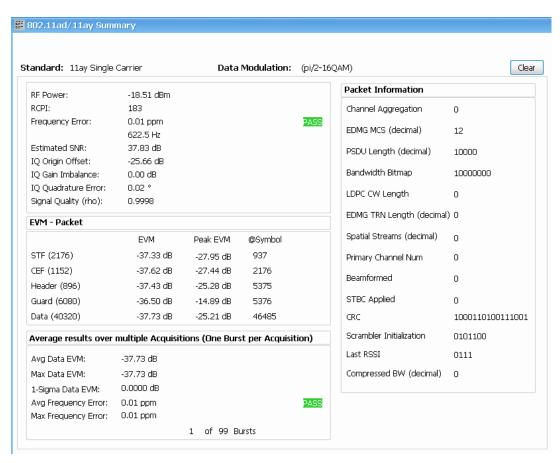
Figure 58: The above image shows an 802.11ad Single Carrier signal with pi/2 16QAM data modulation
