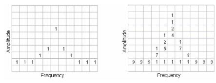
Figure 8: Example 3-D Bitmap Database after 1 (left) and 9 (right) updates. Note that each column contains the same total number of "hits".
