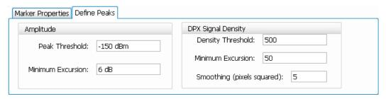
Figure 27: DPX Density control panel is used to define the area of interest for DPX density measurements.
