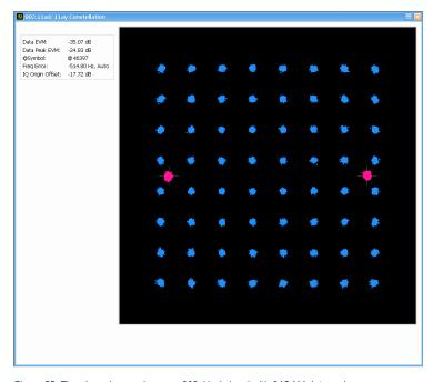
Figure 55: The above image shows an 802.11ad signal with 64QAM data region
