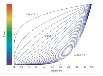
Figure 12: Representative color mapping curves for the "Temperature" palette.
