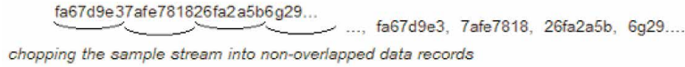
Figure 9: Samples are segmented into data records for FFT processing based on the selected resolution bandwidth.
