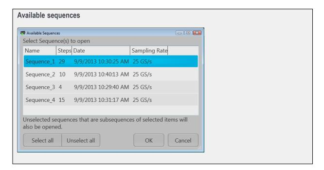
**NOTE.** When opening an AWG70000A Series setup file (.AWGX) from the Waveforms or Sequences tabs, only waveforms and sequences are extracted; instrument settings contained in the setup file are not restored. Use the Open Setup in the File menu to restore the settings, waveforms, and sequences from a .AWGX setup file.
