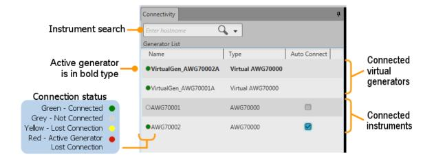
When SourceXpress is started for the first time, one Virtual generated is created and appears in the Generator List as the active generator along with the simulated display of the generator.
