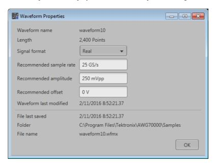
The Waveform Properties dialog screen provides many details about the waveform that are static (not able to modify). The items you are able to modify include:
