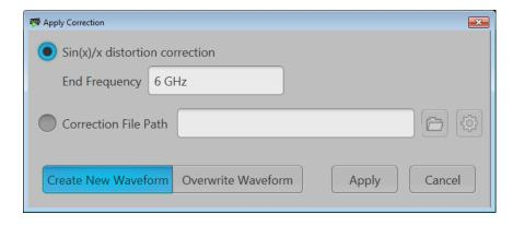
Choose to either create a new waveform or overwrite the existing waveform and select Apply.
