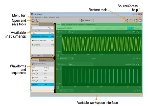
This shaded area of the display is dependant on the type of instrument selected as the active generator.
