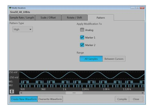
The pattern editor allows you to modify the Analog waveform and/or the Markers. Once you've defined your changes, you need to compile the new waveform. By default, a new waveform is created (based on the existing name) and is placed in the Waveform List.
