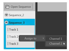
■ Use the drop-down list in the channel's plot area to assign the channel to play a sequence track. You can choose sequence tracks from sequences already loaded into the Sequences tab or you can browse for sequence files. When browsing, you select the sequence file, and then select the track to assign to the channel.
