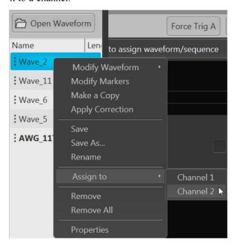
Use the drop-down list in the channel's plot area to assign the channel to play a waveform.
