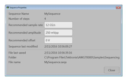
The Sequence Properties dialog screen provides many details about the Sequence that are static (not able to modify). The items you are able to modify include:
