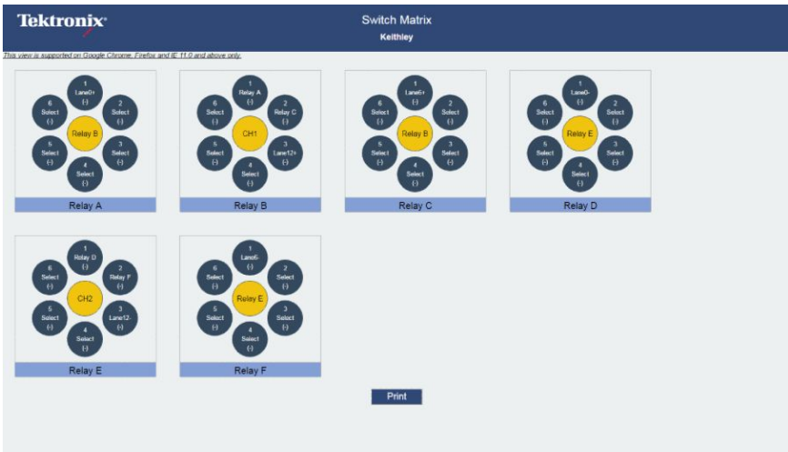
Figure 2: Graphical view of relay cascade configuration
