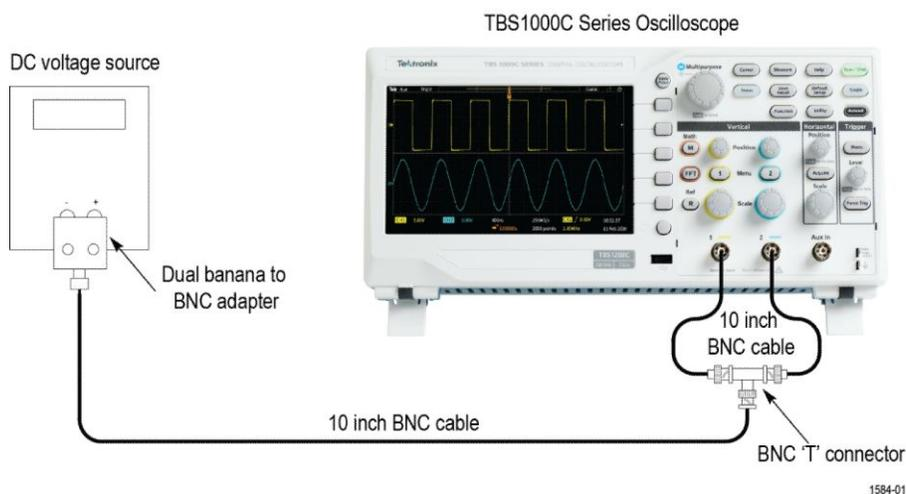
Figure 1: DC voltage setup 1
