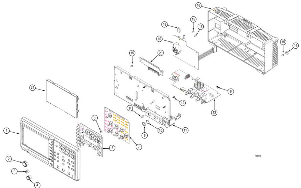
**Table 6: Replaceable parts — (LCD, Front panel, Front case, Power supply, Main board, and Rear case)**
