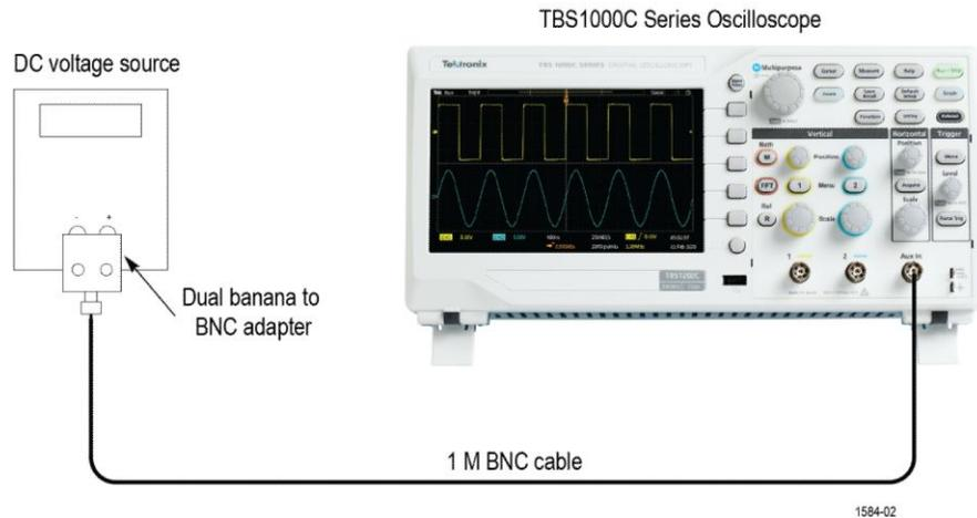
Figure 2: DC voltage setup 2
