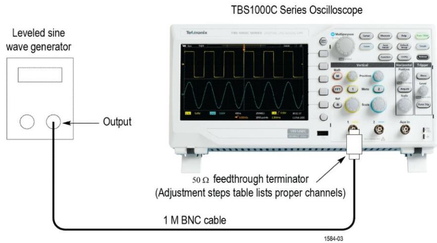
Figure 3: Sinewave generator setup
