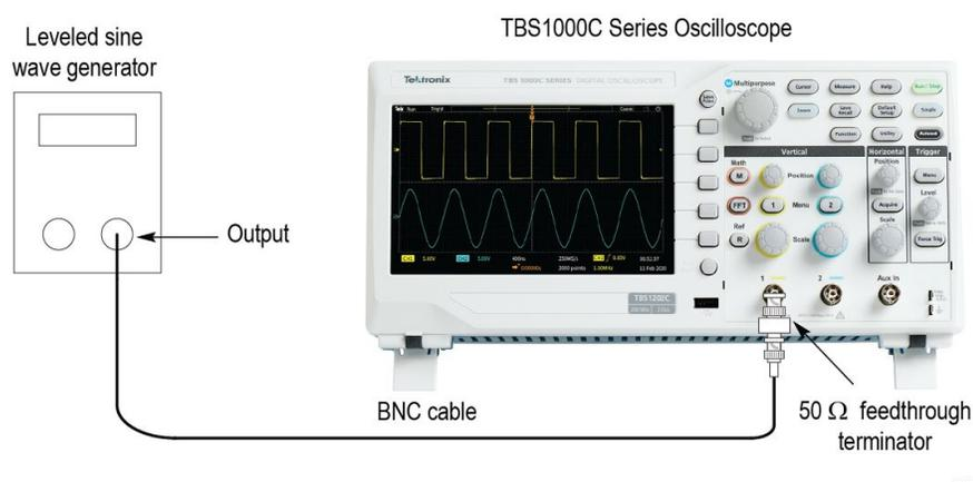
3. Set the oscilloscope **Vertical Scale** (volts/division) to **500 mV/div**.
