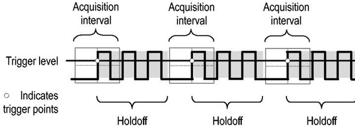
Triggers are not recognized during holdoff time.
