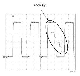
The oscilloscope can respond to an anomalous waveform by stopping acquisitions, emitting a beep, saving the anomalous waveform to a USB flash drive file, printing the screen image to a hard copy device, or any combination of the above. You can also select to highlight just the anomalous data in a waveform, or the entire anomalous waveform.
