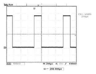
3. Adjust the horizontal Scale to a faster time base setting and increase the Waveform Intensity to see the jitter in the pulse width.
