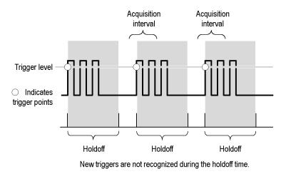
**NOTE.** For best results, choose Normal trigger mode when using long holdoff settings (10 ms or greater).
