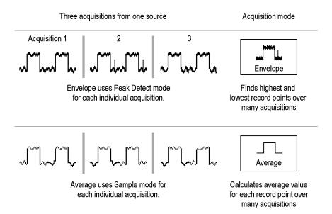
**Envelope.** Use Envelope acquisition mode to capture the minimum and maximum extremes of a signal over a specified number of acquisitions (N). The enveloped waveform data acquisition clears and then starts over after each N acquisitions. If you push the Single Seq button, envelope acquisition stops after N acquisitions. Use the general purpose knob to set the number of acquisitions.
