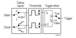
Menu Push the Trigger Menu button, and then push the Type bottom screen button to select Logic. The next table lists the menu items when the trigger Type is set to Logic, and the Class is set to State.
