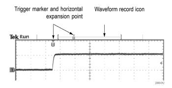
The small inverted triangle is the horizontal expansion point. When you change the horizontal Scale setting, the waveforms contract or expand about this point. When delay is off, the horizontal expansion point is the same as the trigger point.
