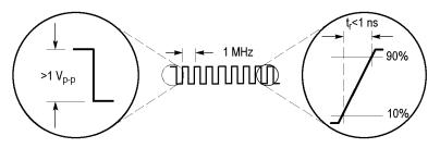
Connect the P3010 to the signal source to display a 1 MHz test signal on your oscilloscope. Use the BNC-to-probe tip adapter (013-0277-00) to make the connection. The oscilloscope should display a waveform similar to the one shown next.
