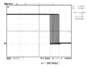
You can also measure the minimum and maximum pulse widths. When you select the first cursor, the @ readout displays the minimum pulse width (210  $\mu$ s). When you select the second cursor, the @ readout displays the maximum pulse width (211  $\mu$ s).
