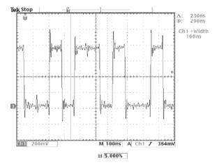
When gating is off, the oscilloscope takes measurements over the entire waveform record.
