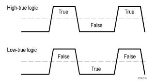
**Boolean Logic.** The signal logic (threshold level and high-true/low-true logic) defines which part of a waveform cycle is true or false. You then use Boolean logic to evaluate or compare the logic of two signals as part of a trigger condition.
