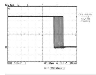
**NOTE.** You can toggle the delay function on and off to view signal details at two different areas of interest.
