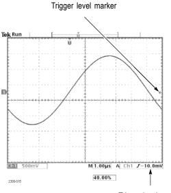
Trigger level readout
