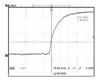
**Measuring Specific Events.** Next you want to see the pulses in the incoming digital signal, but the pulse widths vary so it is hard to establish a stable trigger. To look at a snapshot of the digital signal, follow this step:
