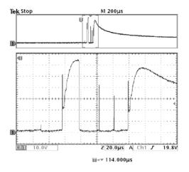
The zoom function works equally well when acquisition is running or is stopped. Horizontal position and scale changes affect only the display, not the next acquisition.
