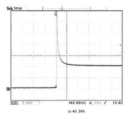
The Single Seq button sets trigger parameters to the correct settings for a single-shot acquisition.
