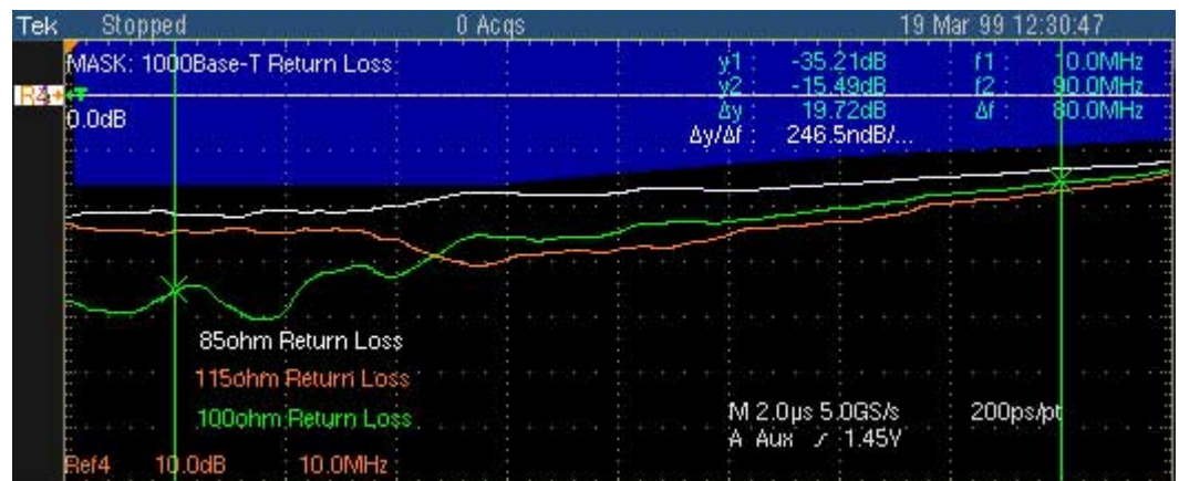
Figure 8-23: Waveform for 1000BASE-T Return Loss
