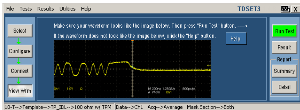
Figure 13-3: 10BASE-T View Waveform for TP_IDL with TPM
