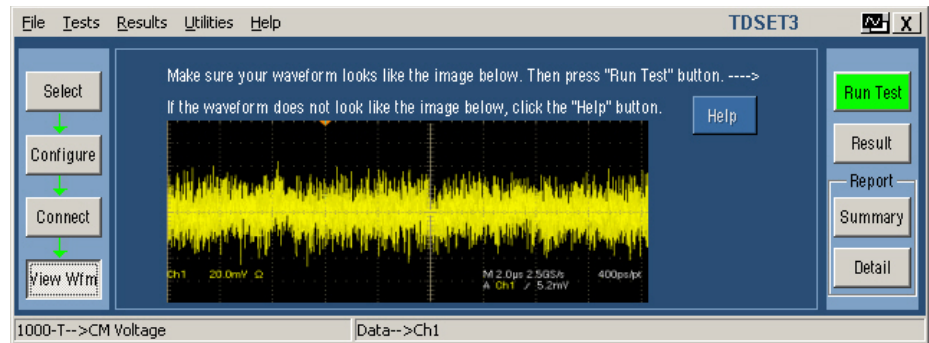
Figure 11-13: 1000BASE-T View Waveform for CM Voltage
