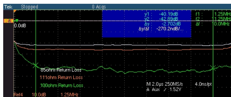
Figure 10-24: Waveform for 10BASE-T Return Loss Receiver
