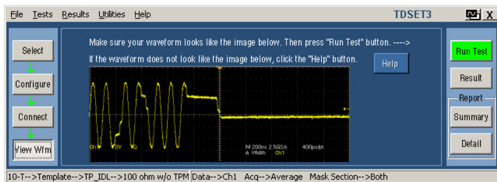
Figure 13-4: 10BASE-T View Waveform for TP_IDL without TPM
