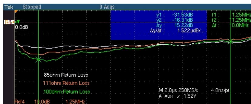
Figure 10-23: Waveform for 10BASE-T Return Loss Transmitter
