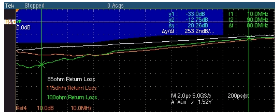
Figure 9-18: Waveform for 100BASE-TX Return Loss Transmitter
