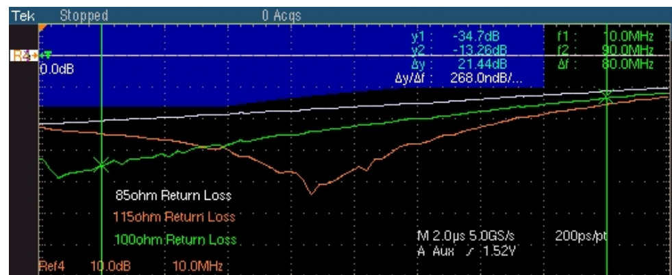
Figure 9-19: Waveform for 100BASE-TX Return Loss Receiver
