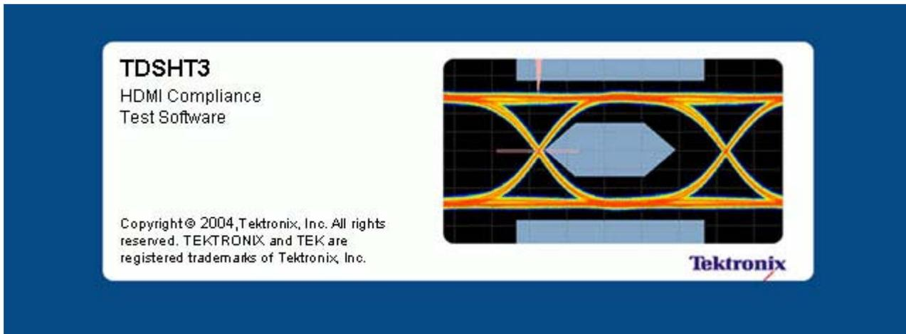
The TDSHT3 HDMI Compliance Test Software is a High Definition Multimedia Interface (HDMI) compliance test solution. This software helps the test, validation, and design engineers perform both HDMI physical layer validation and compliance testing. The TDSHT3 HDMI Compliance Test Software provides credible test results in conformance with the HDMI standards and test specifications.
