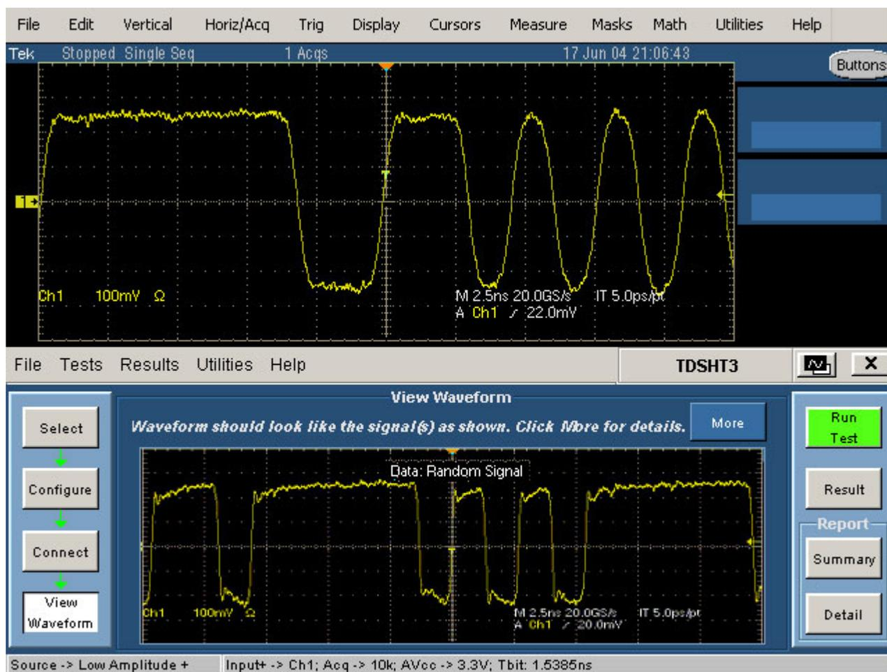
10. If you have selected existing Tbit value, then click **View Waveform** to get a different waveform on your display. Ensure that your signal in the oscilloscope display is similar to the sample signal.
