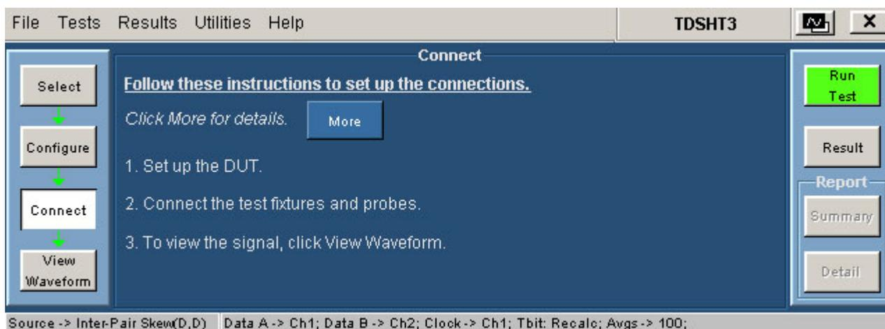
8. Ensure that your signal in the oscilloscope display is similar to the sample signal. Click **View Waveform** to display a sample of the expected signal. If the displays are not similar, go back and check your configuration and connections. The waveform shown here is for the re-calculate Tbit option. Click **Run Test** to run the test. The **Confirm** dialog box appears. Click **Continue** to continue to run the test. Go to step 10.
