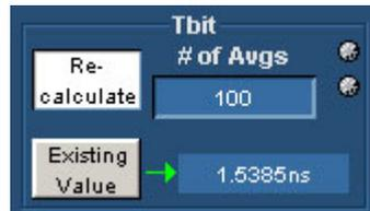
Tbit is the time that is required to transmit one bit of data. Tbit is one bit time at the specified pixel clock frequency ( $= T_{\text{PIXEL}}/10$ ).
