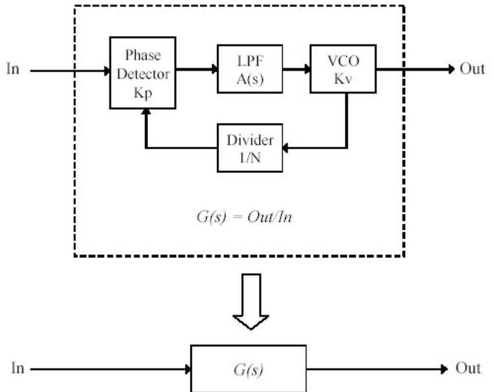
The diagram shows a simplified block diagram of generic phase-locked loop (PLL). A PLL consists of the Phase Detector (PD), Low Pass Filter (LPF), Voltage Controlled Oscillator (VCO), and Frequency Divider (FD).
