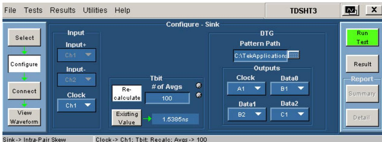
**Note:** The default configuration is to calculate the intra-pair skew of the clock channel. If you want to calculate the intra-pair skew for other data channels, then interchange the DTG physical channels of Data<X> with Clock. For example, to calculate the intra-pair skew of Data0, assign A1 to Data0 and assign B1 to Clock. Make the appropriate changes in the test connections.
