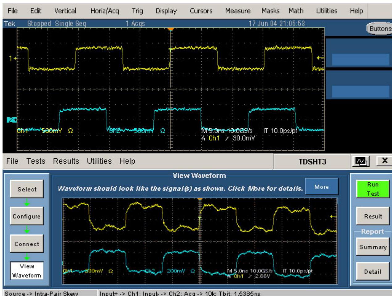
9. If you have selected existing Tbit value, then click **View Waveform** to get a different waveform on your display. Ensure that your signal in the oscilloscope display is similar to the sample signal.
