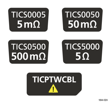
Wideband shunt labels
