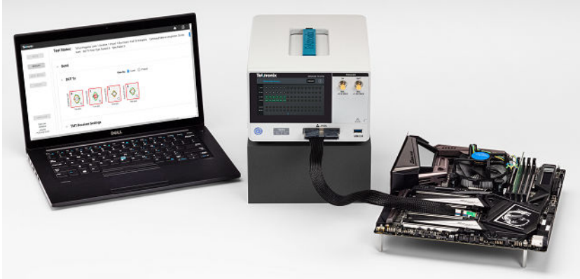
Figure 18: Setup using M.2 Edge adapter and integrated cable for motherboard testing.
