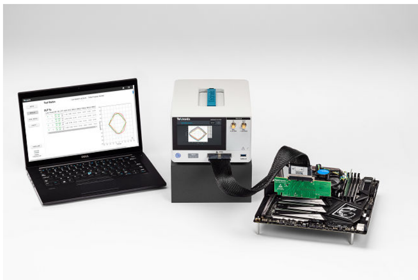
Figure 16: Quick scan setup example using a x16 CEM Edge adapter for motherboard testing. Quick scans can be run and results seen from the front panel and the web UI.
