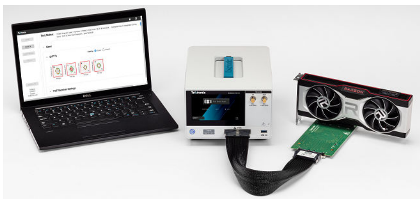
Figure 17: Custom scan setup example using a x16 CEM Slot adapter for graphics card testing. Custom scan can only be run and results seen from the web UI.
