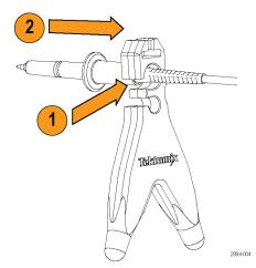
Position the base of the probe holder on your circuit where it can maintain stability while contacting the test point.
