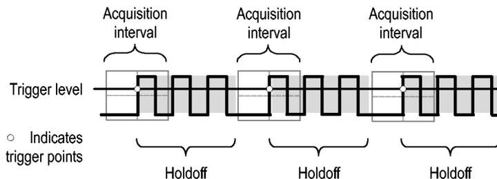
Triggers are not recognized during holdoff time.
