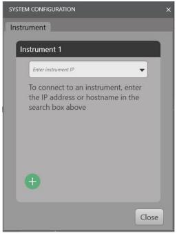
6. Press the green + button (or the Enter key on a keyboard) and the instrument will connect. Mainframe and modules names and firmware versions will appear.
