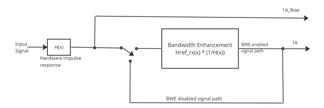
If the user wants to perform measurements on the signal before BWE, then configure MATH with the input source as "channel>\_Raw" and use MATH as the source for measurements.
