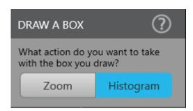
2. If the Histogram icon button is blue, that means the histogram function is on and you can simply draw a box on the waveform to define a new histogram.
