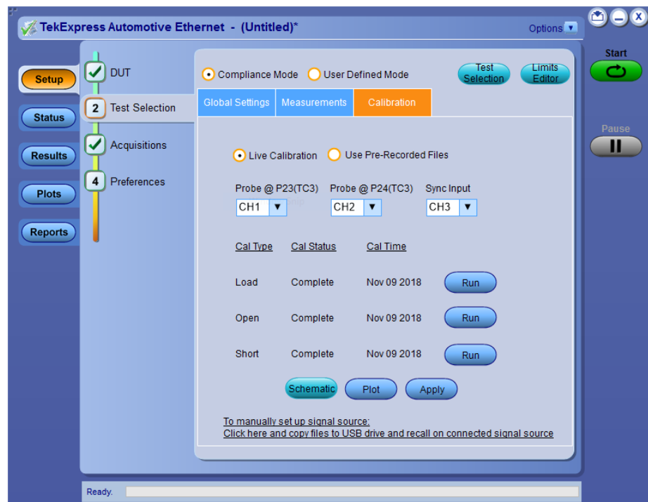
Figure 12: Calibration tab for return loss measurement
