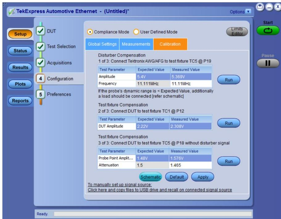
Figure 62: Calibration tab for 100Base-T1 transmitter distortion measurement
