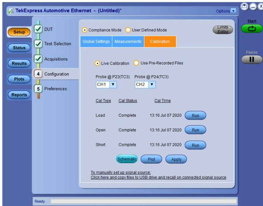
Figure 13: Calibration tab for return loss measurement
