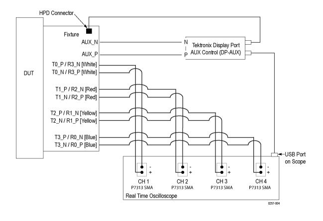
Setup using Tektronix DP-AUX Controller without an RF Switch
