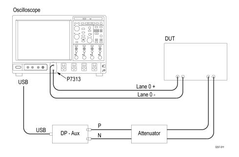
Setup for Aux Channel test
