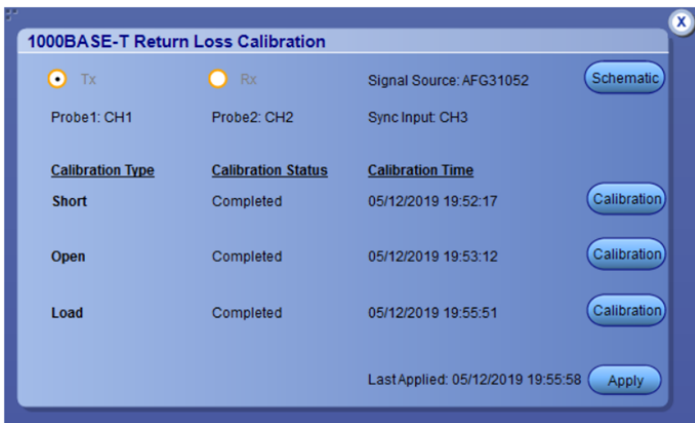
Figure 9: Calibration panel after calibration is performed for OPEN, SHORT, and LOAD and then Apply
