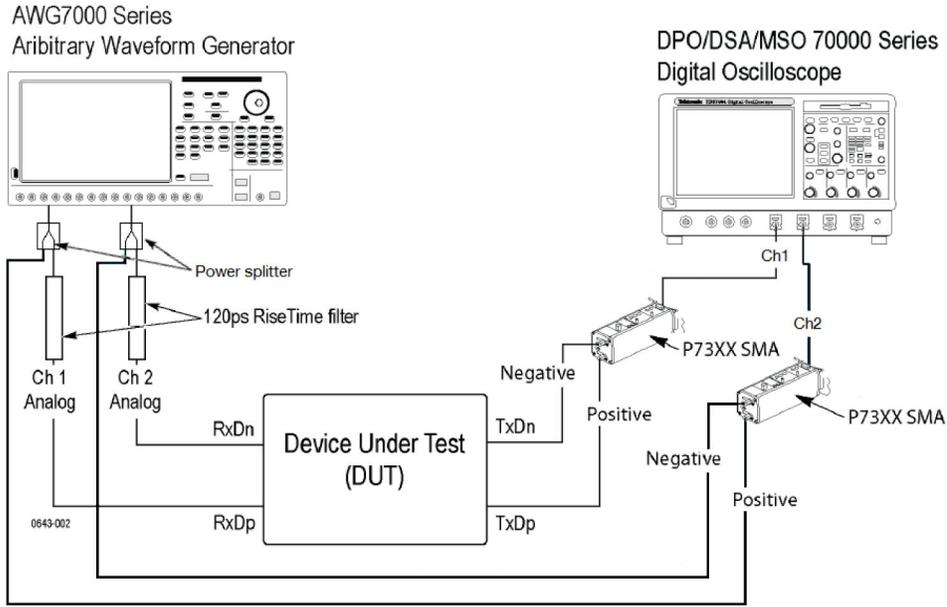
HS Margin schematic for Gear 1 and Gear 2
