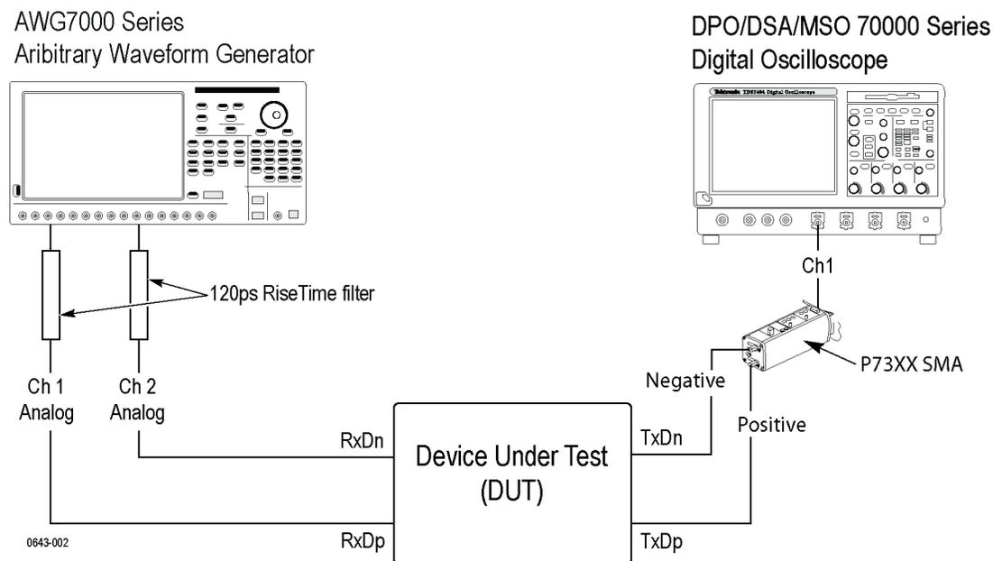
2. Connect the TxDp and TxDn pins of the DUT to the oscilloscope using a matched pair of SMA cables and a differential probe.
