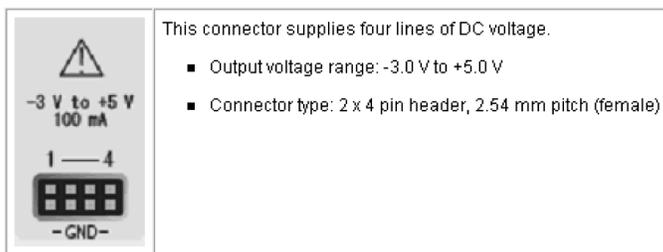
Of these four lines, only the first two DC outputs (DC1 and DC2) are used.
