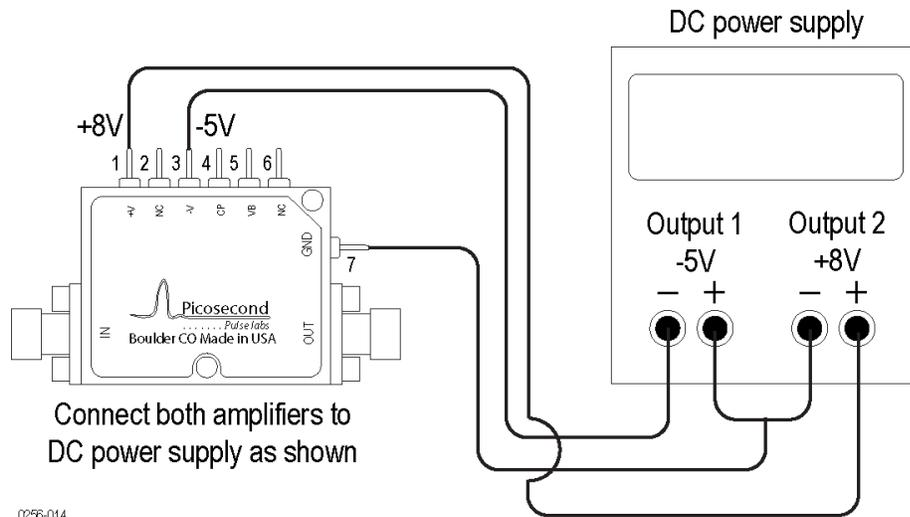
Connect both amplifiers to DC power supply as shown
