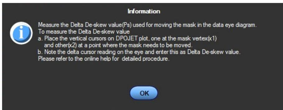
After you select OK, the Measure the Deskew Value pop-up dialog box displays. Once you determine how the amount of time (in pico seconds) to shift the mask horizontally, enter the value here. To determine the amount of deskew time, use the procedure [Moving the Mask \(see page 190\)](#).
