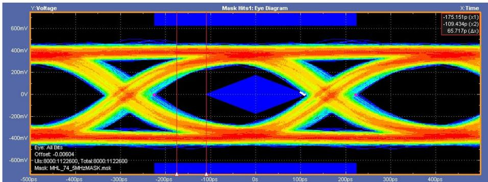
2. Using the delta cursors, measure the amount of time you want to shift the mask. In the example, we've measured that we want to shift the mask -65 ps.
