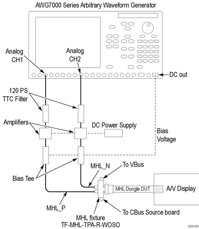
Dongle Min-Max Setup
