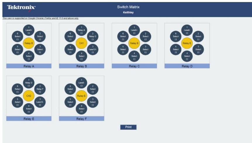
Figure 8: Graphical view of relay cascade configuration
