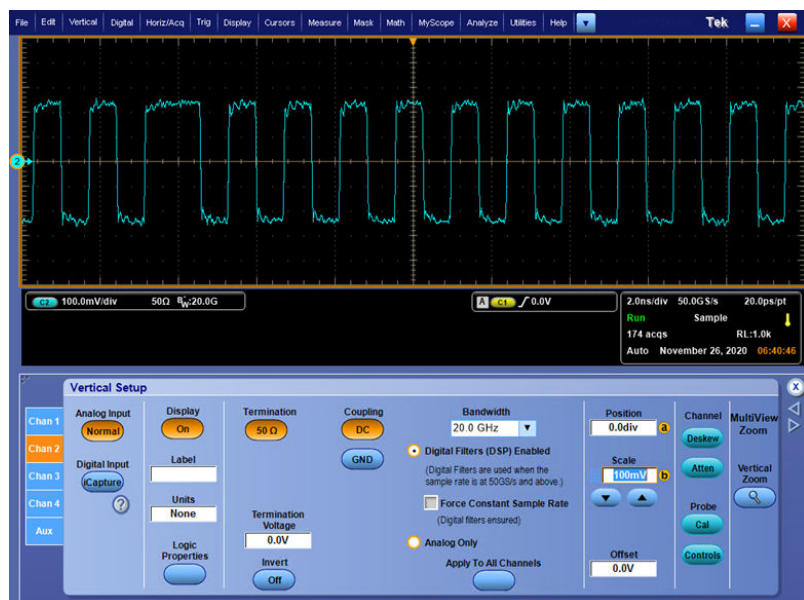
Figure 123: Example for the channel vertical scale configuration
