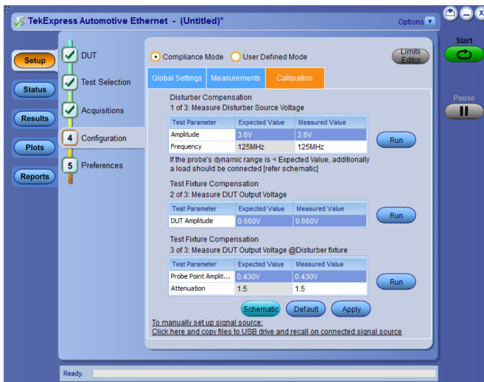
Figure 1: Calibration tab for 1000Base-T1 transmitter distortion measurement
