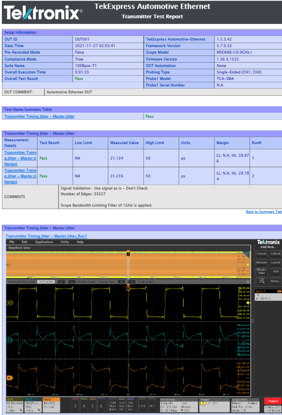
Figure 52: Report of 100/1000Base-T1 probing type Single-Ended
