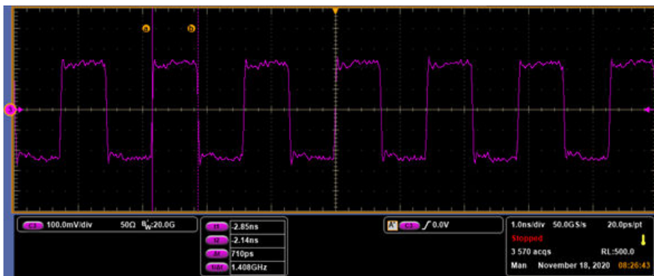
Figure 61: Example TestMode#2, JP03A waveform for 2.5GBASE-T1
