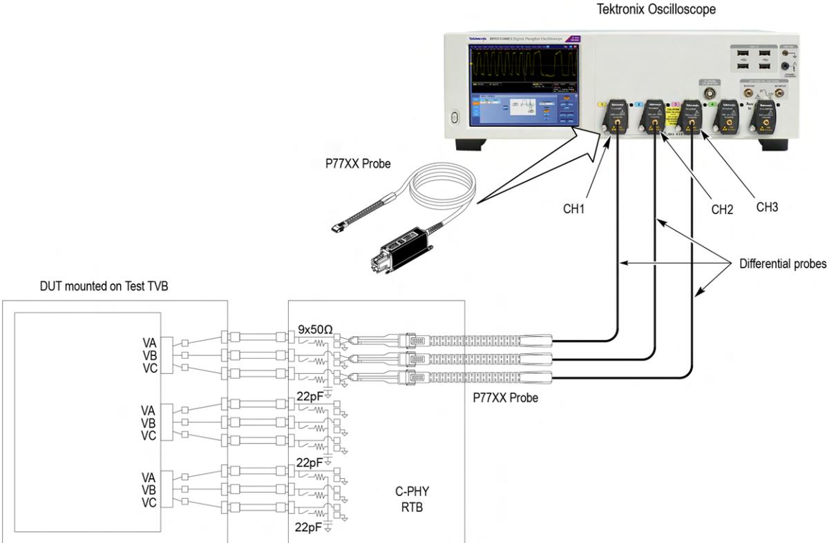
Note: Switch OFF the termination on RTB using dip switch
