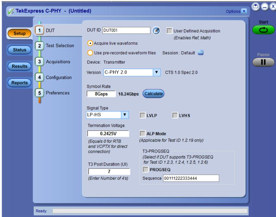
The Tektronix C-PHY Tx 2.0 Automated Test software runs on Tektronix real-time oscilloscopes that are based on Windows 10 computer operating systems. C-PHY Tx 2.0 delivers the TekExpress based C-PHY automation solution with Tx measurement.
