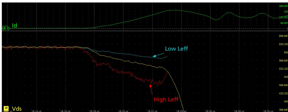
Figure 36: V_{ds} modelled using low L_{\text{eff}} (blue) and high L_{\text{eff}} (red) to match zero skew acquired V_{ds} (yellow) during turn on transient
