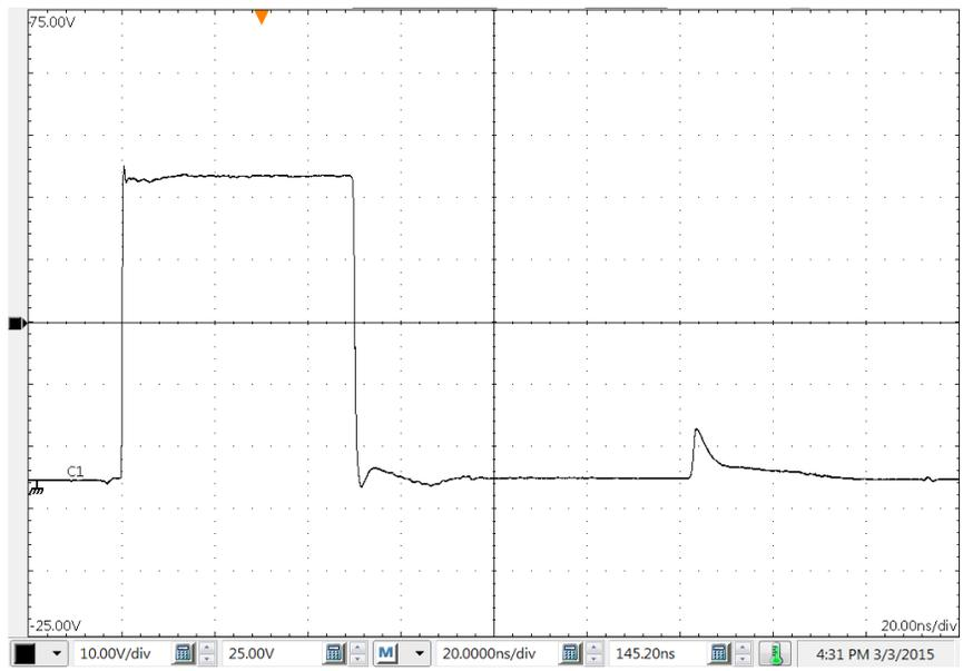
Figure 10: 50 ns duration pulse waveform.
