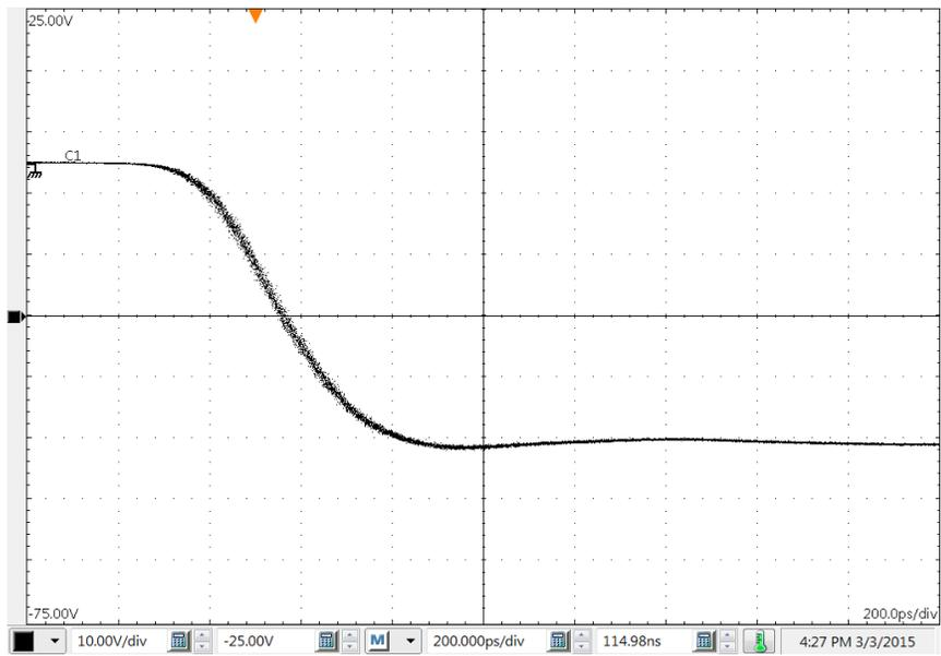
**Figure 8: Trailing edge waveform**
