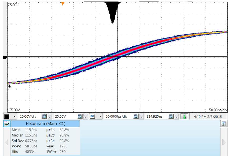
Figure 13: Fixed 115 ns delay trigger, jitter measures 6.8 ps<sub>rms</sub>
