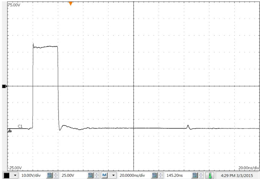
**Figure 9: 20 ns duration pulse waveform**
