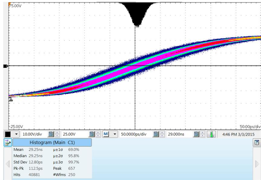
Figure 12: Adjustable delay trigger, jitter measures 12.8 ps<sub>rms</sub>
