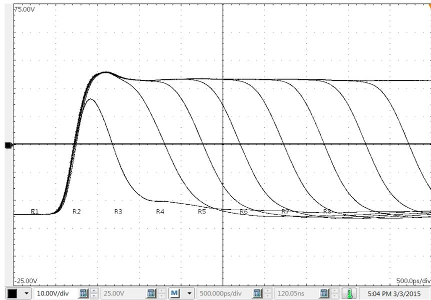
Figure 14: Adjustable duration waveform
