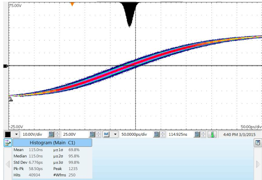
Figure 13: Fixed 115 ns delay trigger, jitter measures 6.8 ps<sub>rms</sub>
