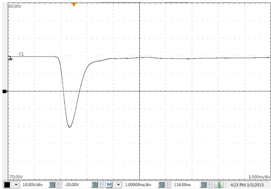
**Figure 6: Minimum duration negative pulse**
