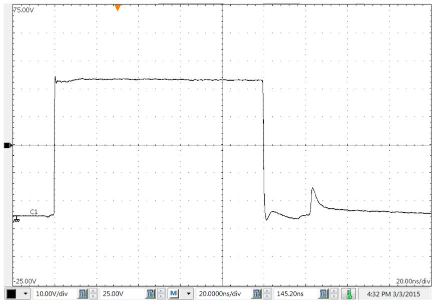
Figure 11: 100 ns duration pulse waveform
