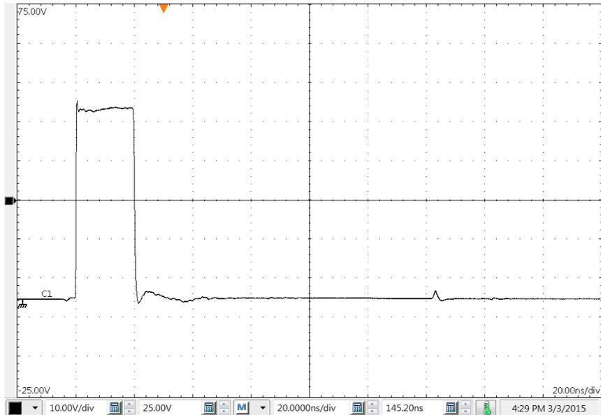
**Figure 9: 20 ns duration pulse waveform**
