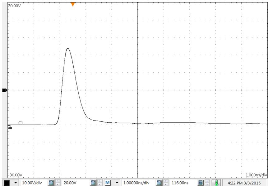
**Figure 5: Minimum duration positive pulse**
