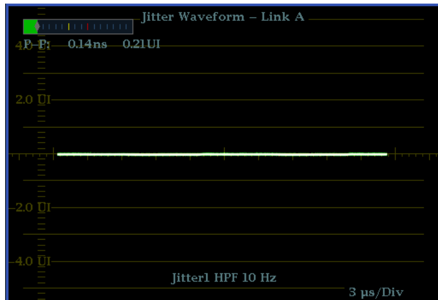
Figure 25: The Jitter display parameters as shown in a single tile when the instrument is in 4-tile mode
