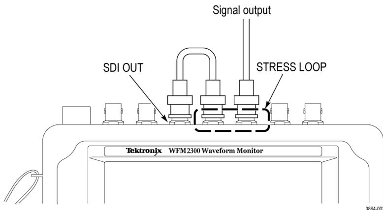
**Figure 4: Stress loop connections for a generated signal**
