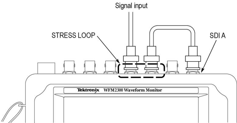
**Figure 3: Stress loop connections for a monitored signal**
