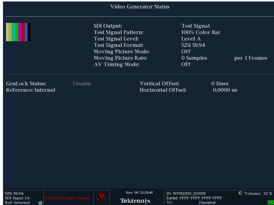
Figure 51: Video Generator Status display
