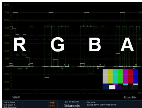
Figure 7: Placement of dual link information in the Waveform display
