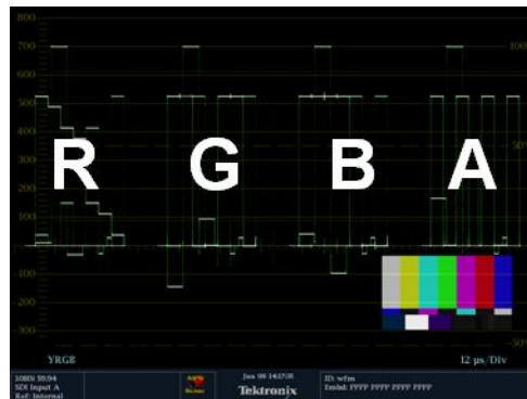
Figure 7: Placement of dual link information in the Waveform display
