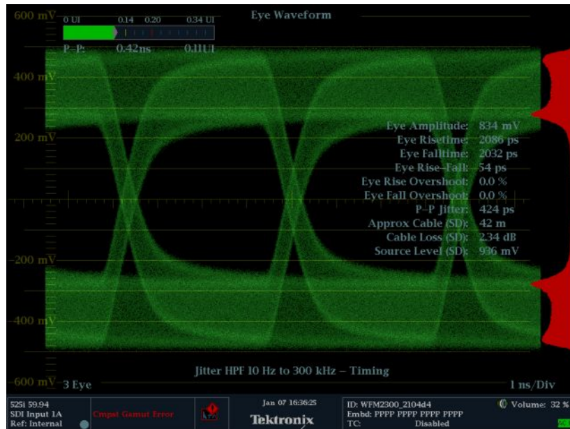
Figure 25: WFM2300 Eye display in single tile mode (full-screen) with histogram
