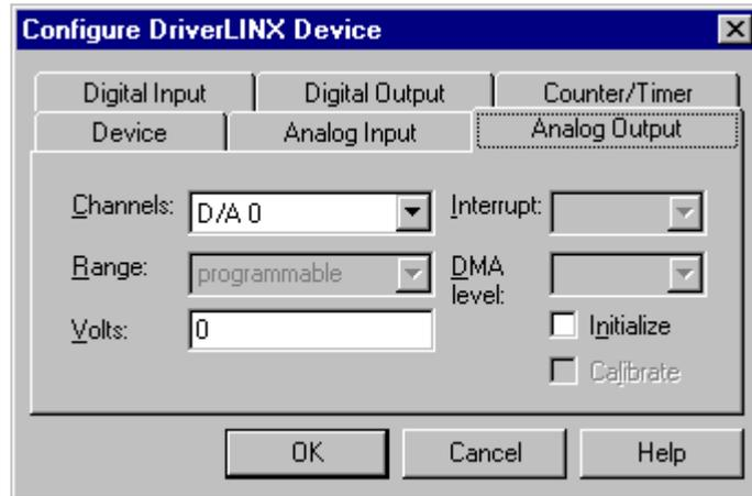
Use the Analog Output subsystem page to set or view the initial output voltages.
