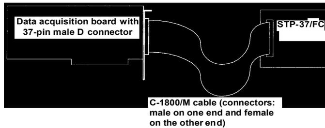
Figure 2. Connecting the STP-37/FC to the data acquisition board
