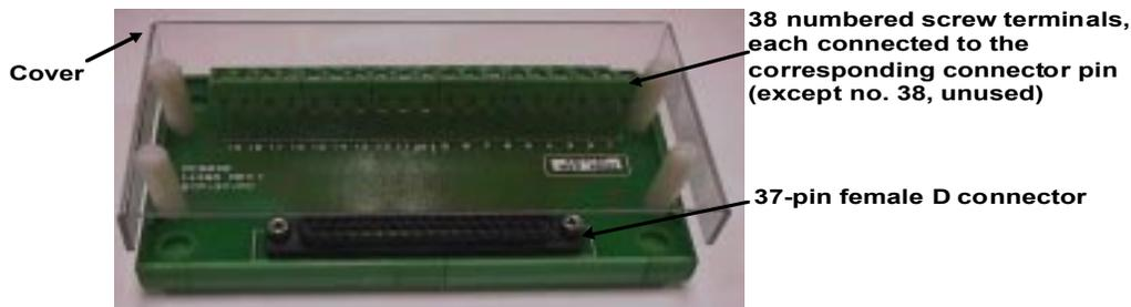
Figure 1. Layout of STP-37/FC screw terminal panel
