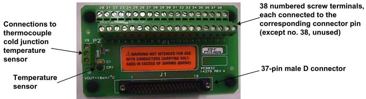
Figure 1. Layout of STP-37 screw terminal panel
