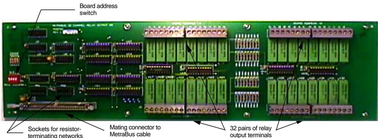
The board address setting is the sum of the numbers set to ON at the board address switch (i.e., the number 4, 8, 16, or 32 printed above an individual DIP switch pole indicates the number that is added to the address when that pole is turned to ON). For example, to set a board address of 20, turn switch poles numbered 4 and 16 to ON and turn the other poles to OFF. See Figure 2.
