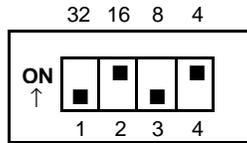
**Figure 2. Setting a board address of 20**
