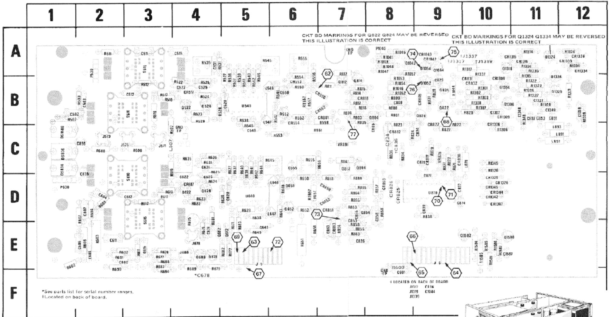
Fig. 8-12. A8—Trigger Generator and Sweep Logic circuit board.
