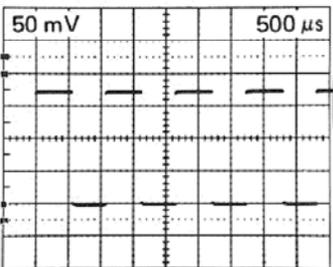
For waveforms 11 through 15. Connect the calibrator signal to the CH 2 input via a X10 probe. Set the VERT MODE switch to CH 2.
