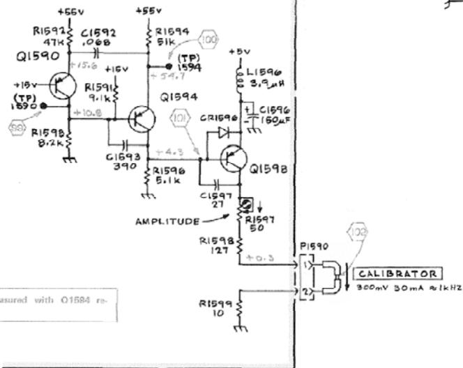
Voltages measured with Q1584 removed
