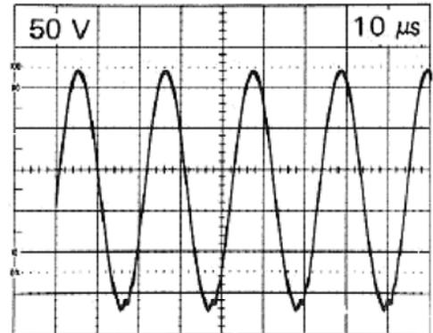
The amplitude of this waveform varies from 0 volts to 75 volts peak-to-peak depending on the setting of the Intensity control.
