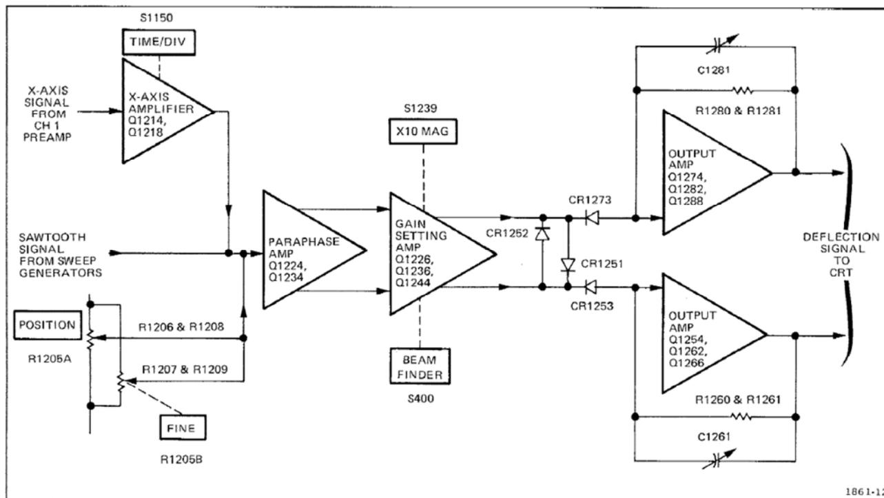
Fig. 3-7. Detailed block diagram of the Horizontal Amplifier.
