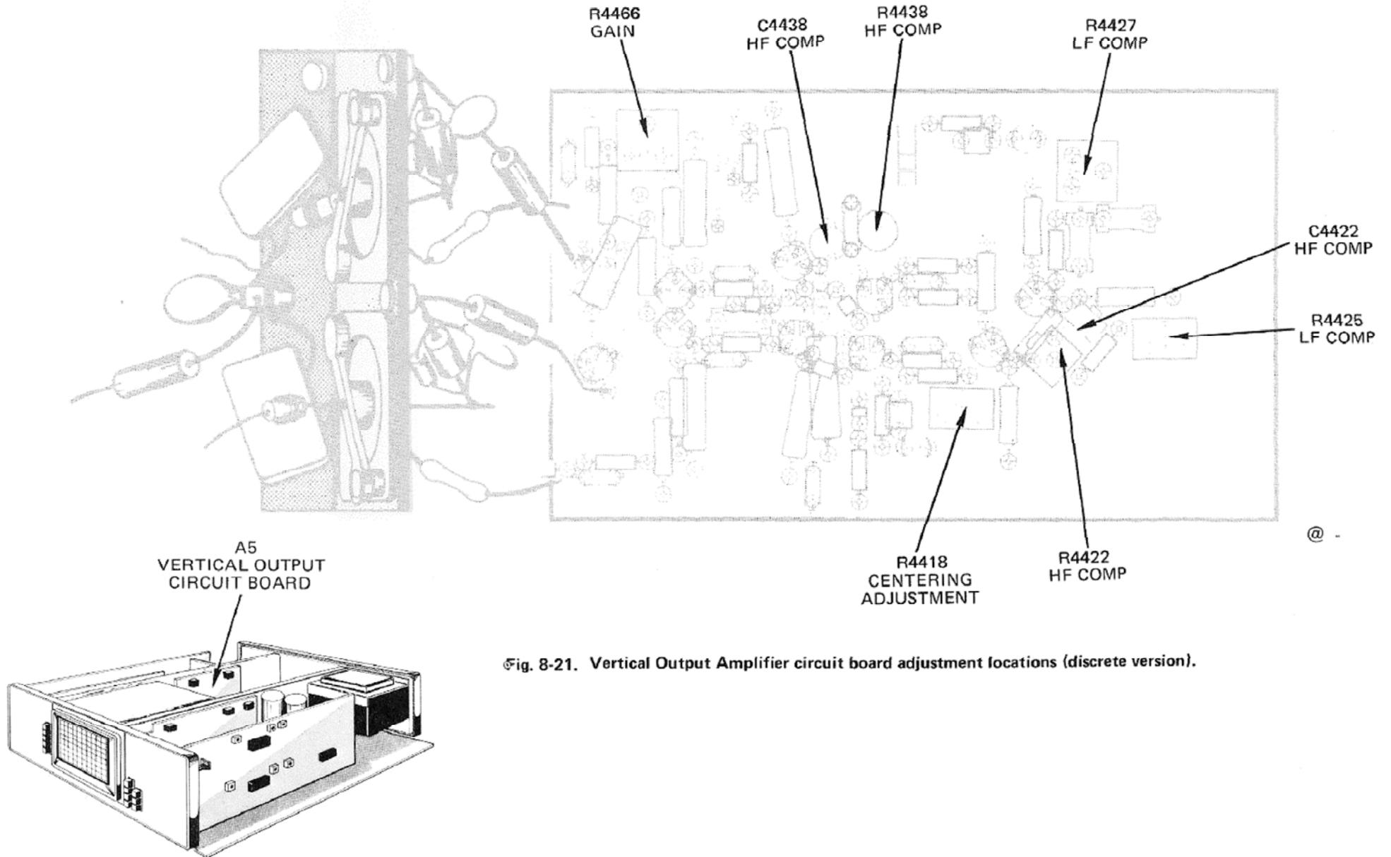
Fig. 8-21. Vertical Output Amplifier circuit board adjustment locations (discrete version).
