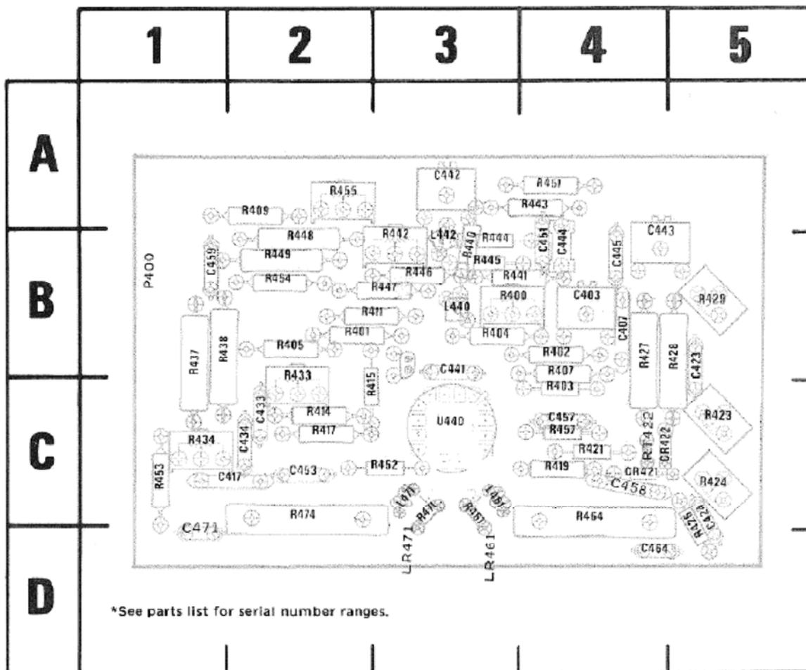
Fig. 8-8. A5b—Vertical Output Amplifier circuit board (IC version).
