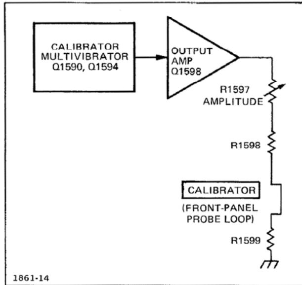
Fig. 3-9. Detailed block diagram of the Calibrator circuit.
