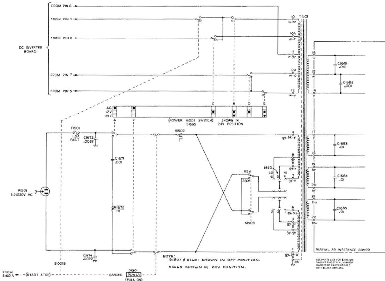
Fig. Option 7-3. 465 Option 7 primary winding.
