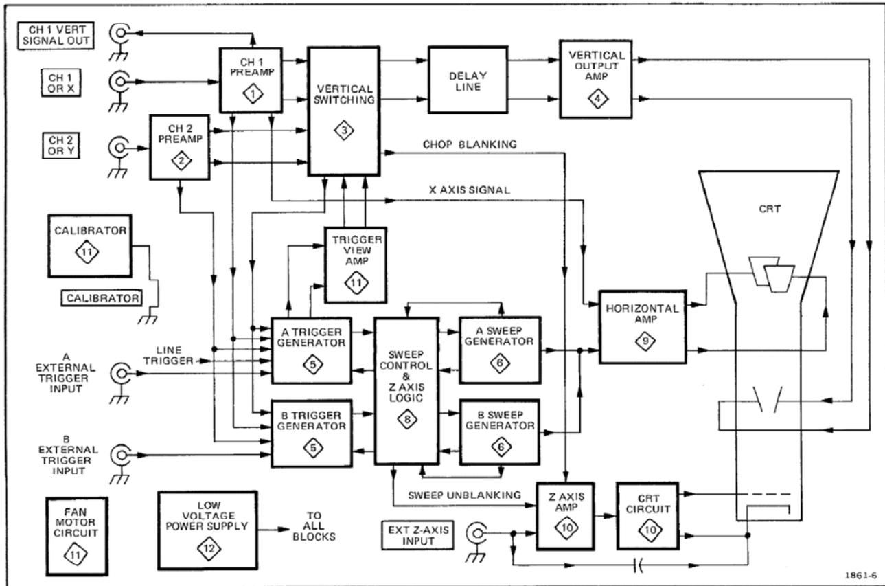
Fig. 3-1. Basic block diagram of the 465.
