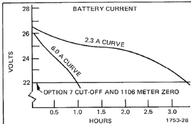
Fig. Option 7-4. Typical battery pack discharge curves.
