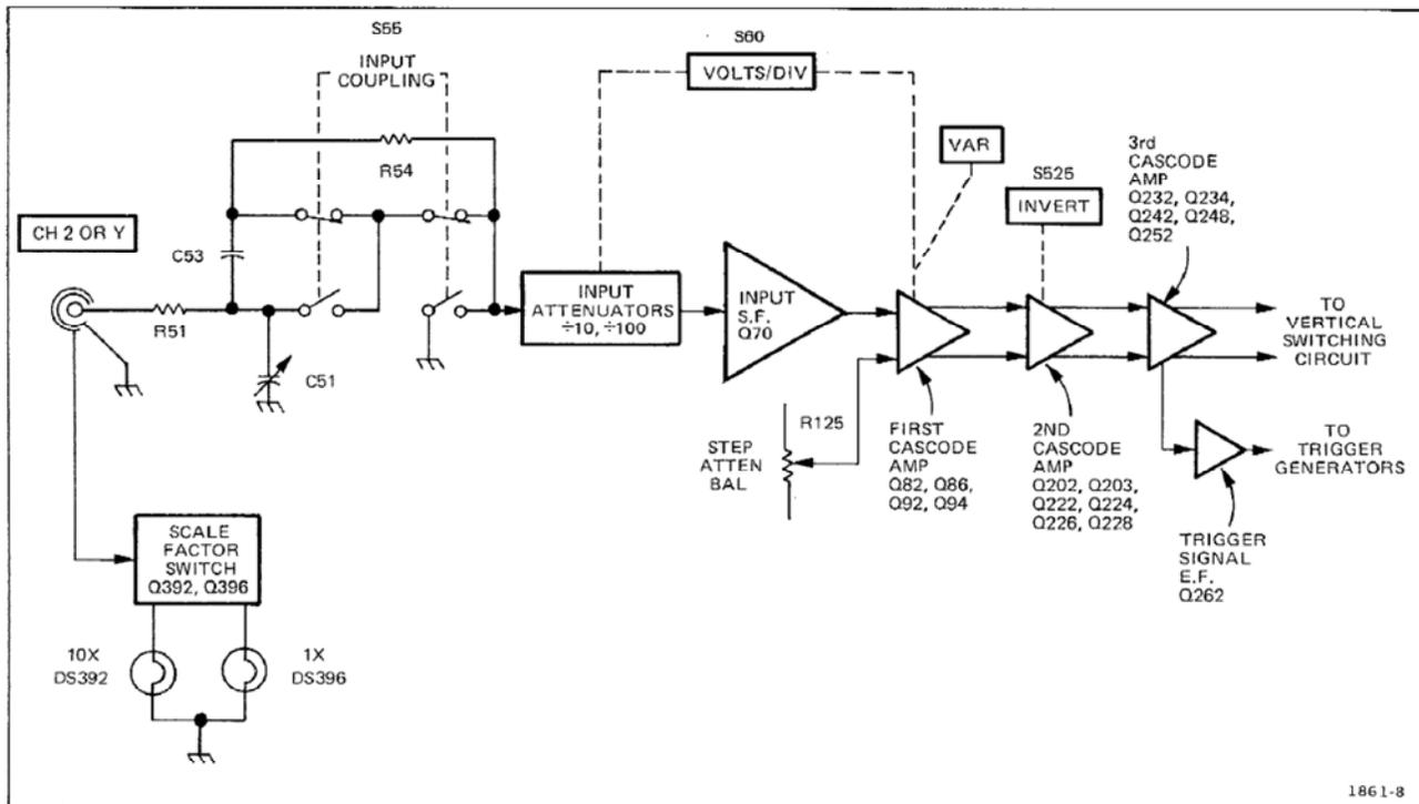
Fig. 3-3. Detailed block diagram of the Channel 2 Preamplifier.
