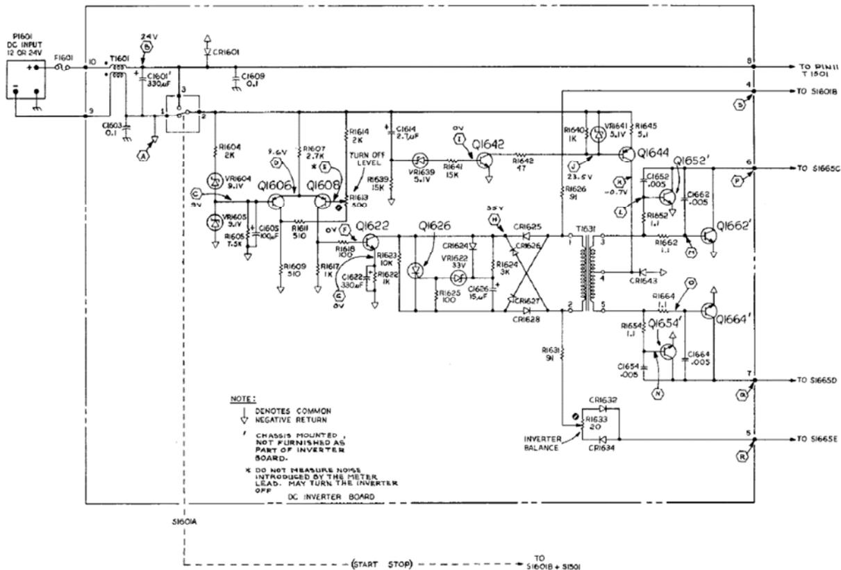
Fig. Option 7-2. 465 Option 7 DC Inverter.
