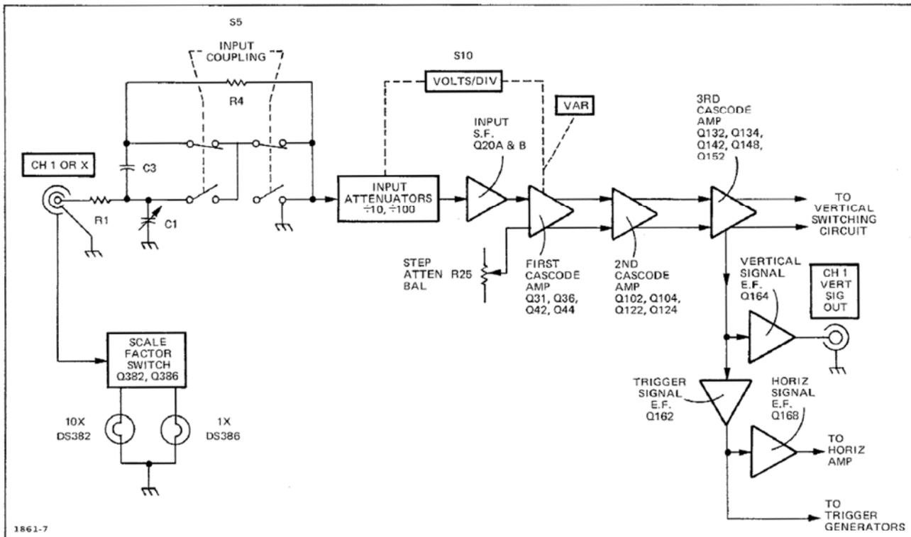
Fig. 3-2. Detailed block diagram of the Channel 1 Preampifier.
